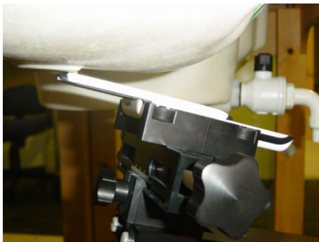
DUT position towards the head Slider Open: Tilt (touch + 15°) position
