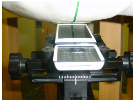
DUT position towards the head Slider Open: Tilt (touch + 15°) position
