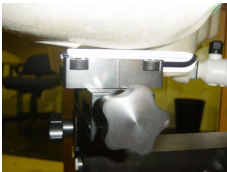
DUT position towards the head Slider Closed: Cheek and Tilt (touch + 15°) positions
