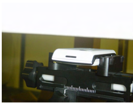
DUT position towards the body with Slider Closed and 15 mm distance
