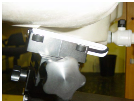
DUT position towards the head Slider Closed: Cheek and Tilt (touch + 15°) positions
