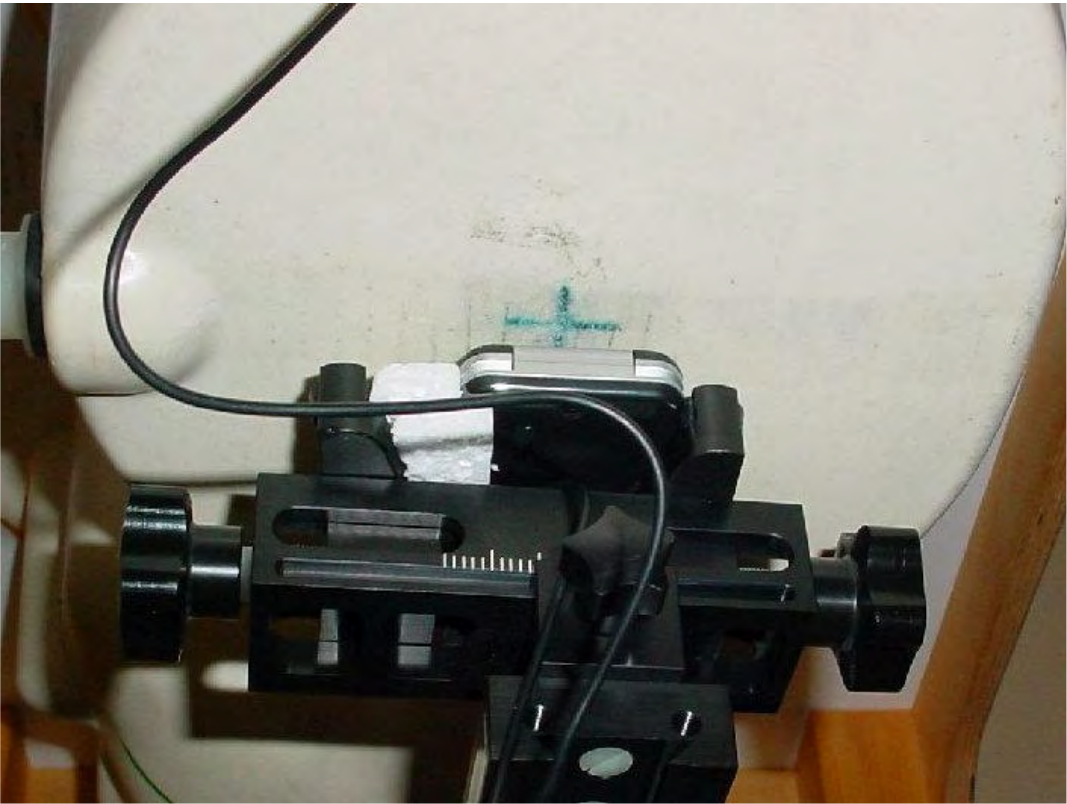
Photo 25: Test position body worn front side with 15 mm distance
