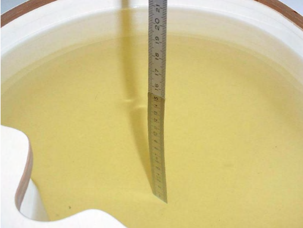
Photo 27: Liquid depth 850 MHz body simulating liquid
