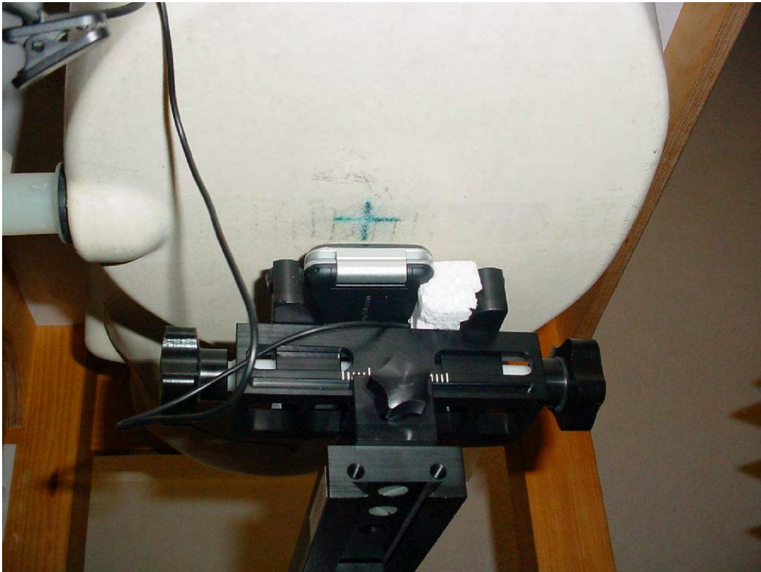
Photo 24: Test position body worn front side with 15 mm distance
