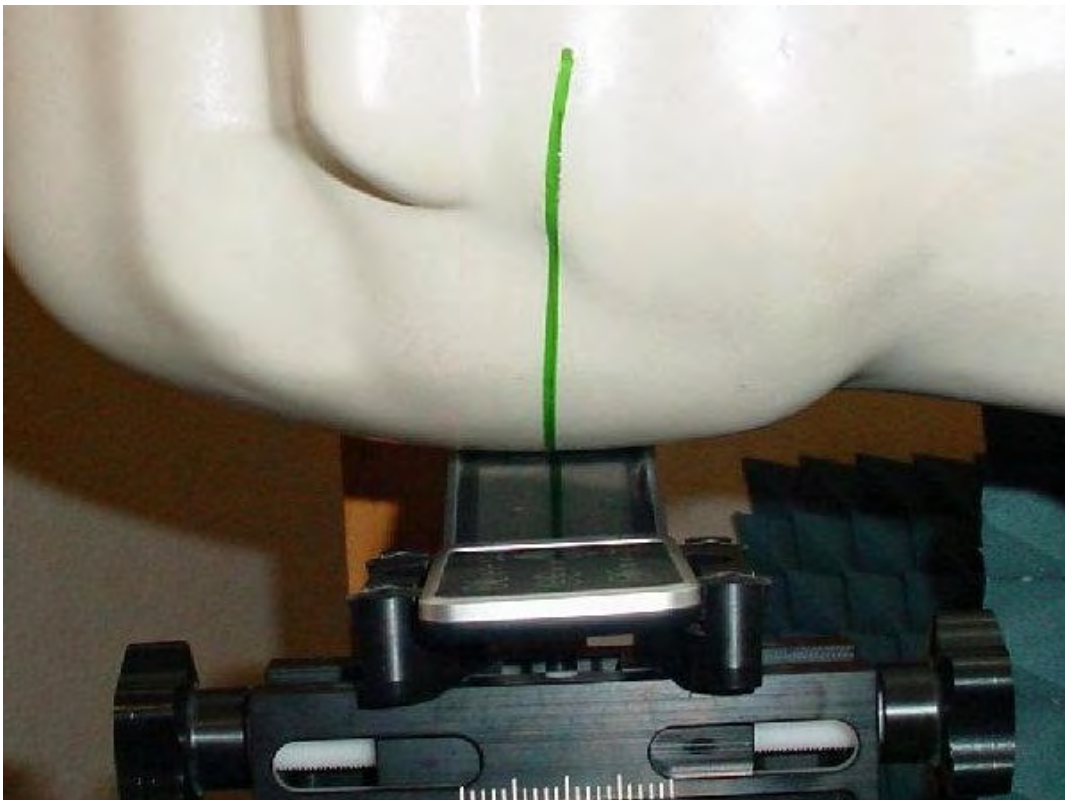
Photo 20: Test position right hand tilted 15°
