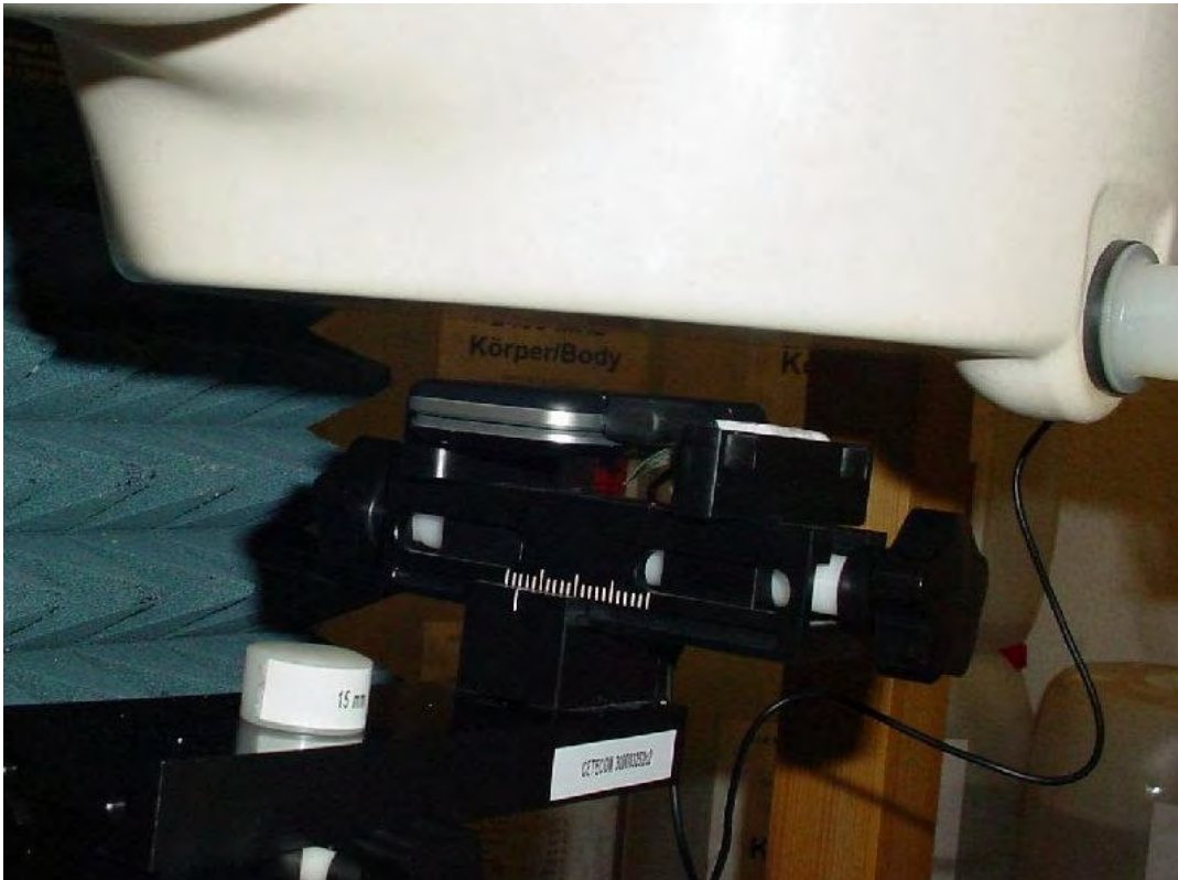
Photo 24: Test position body worn front side with 15 mm distance
