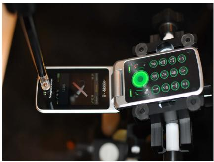
Figure 13-1 Test Setup for Wireless Device
