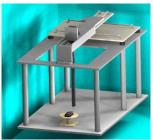
Figure 5-3 RF Near-Field Scanner
