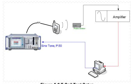
Figure 5-2 T-Coil Test Setup
