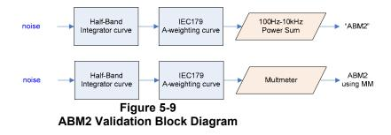
The power summed output results for a known input were compared to the multi-meter results to verify any deviation in the post-processing implemented with the power-sum.
