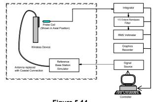
Figure 5-14 Audio Magnetic Field Test Setup
