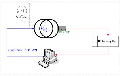
Figure 5-1 Validation Setup with Helmholtz Coil
