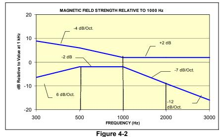
Magnetic Field frequency response for wireless devices with an axial field that exceeds –15 dB(A/m) at 1 kHz
