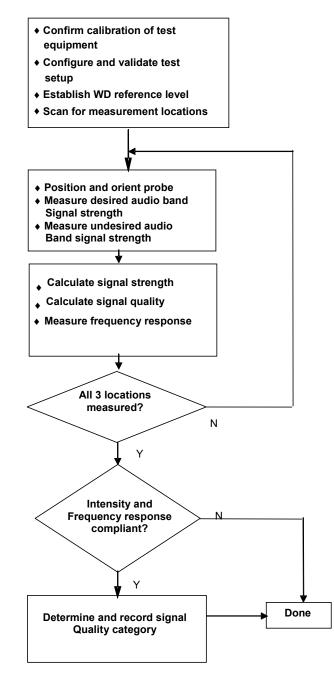
Figure 5-16 C63.19 T-Coil Signal Test Process
