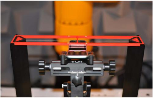
Figure 17-2 HAC Phantom Plane Alignment
