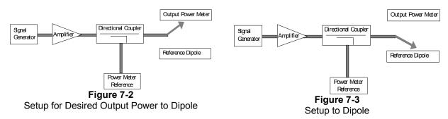
Using this setup configuration, the signal generator was adjusted for the desired output power (100mW) at a specified frequency. The reference power from the coupled port of the directional coupler is recorded. Next, the output cable is connected to the reference dipole, as shown in Figure 7-3.
