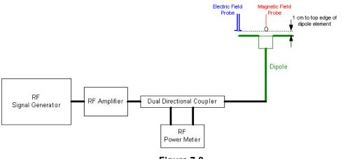
Figure 7-8 System Check Setup
