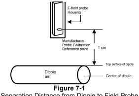
Separation Distance from Dipole to Field Probe
