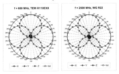
Receiving Pattern ( $\phi$ ),  $\vartheta = 0^{\circ}$
