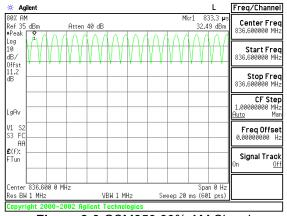
Figure 8-3 GSM850 80% AM Signal
