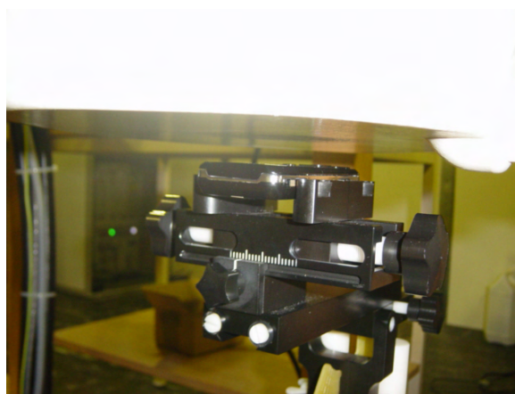
DUT in body position with 15 mm distance
