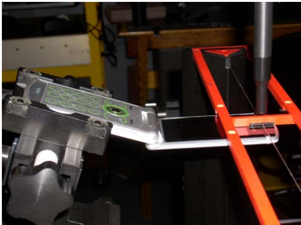
Figure 17-2 HAC Phantom Plane Alignment
