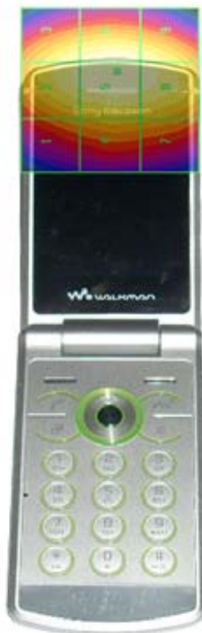
Figure 17-4 E-Field WD Scan overlay
