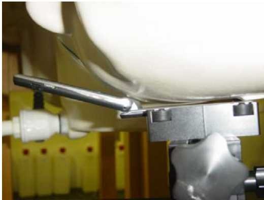
DUT position towards the head Flip Open: Cheek (touch) position
