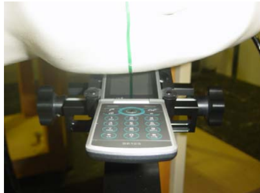
DUT position towards the head Flip Open: Tilt (touch + 15°) position
