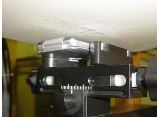
DUT position towards the body with Flip Closed and 15 mm distance
