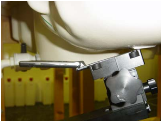
DUT position towards the head Flip Open: Tilt (touch + 15°) position
