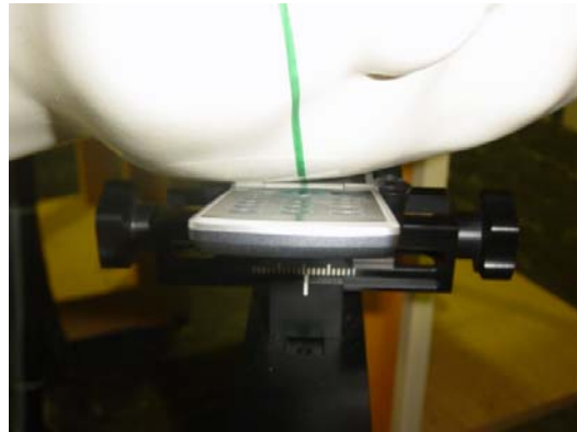
DUT position towards the head Flip Open: Cheek (touch) position
