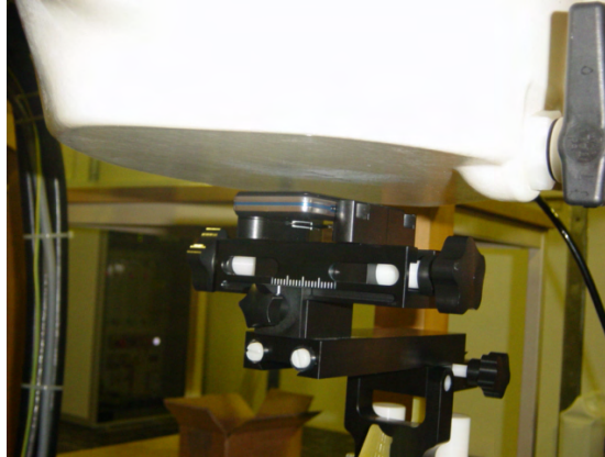
DUT in body position with 15 mm distance
