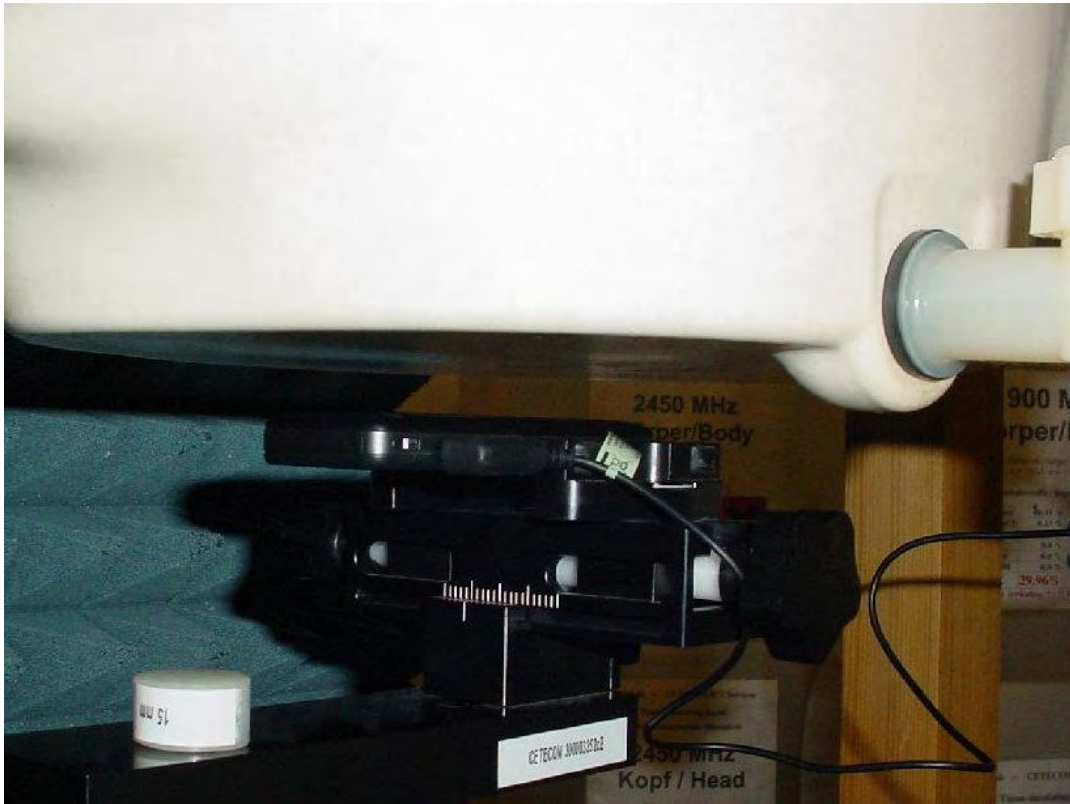
Photo 22: Test position body worn rear side with 15 mm distance
