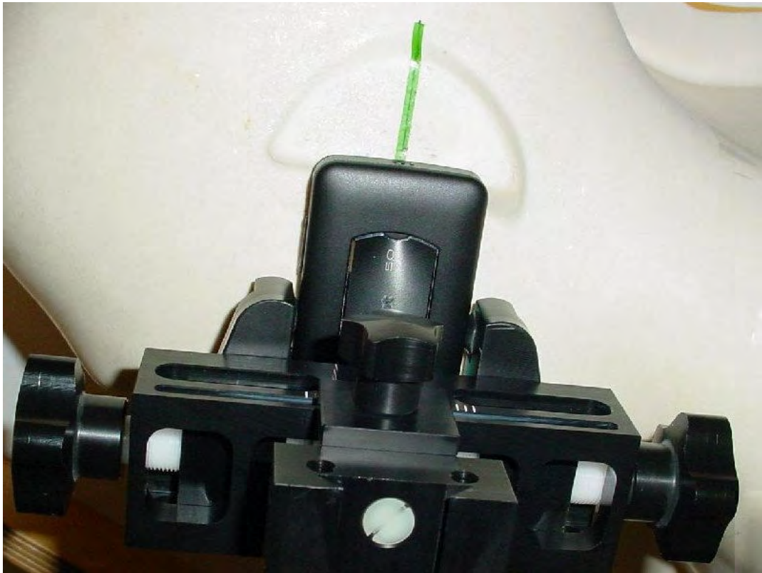
Photo 12: Test position left hand tilted 15°
