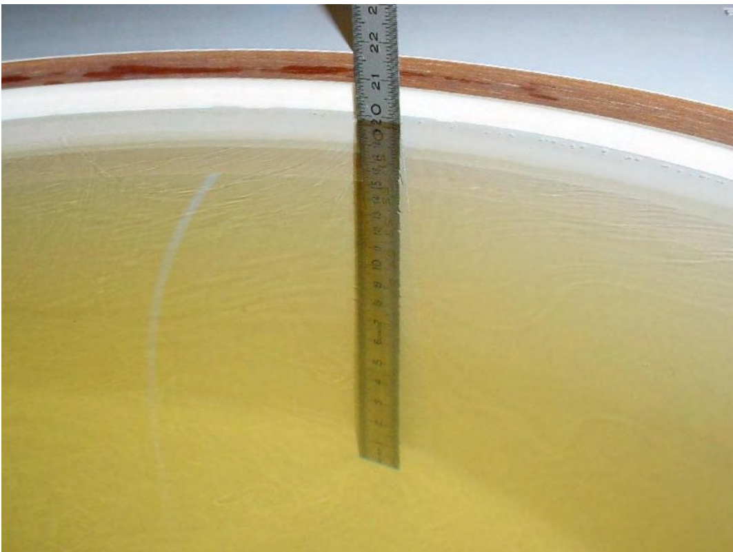
Photo 24: Liquid depth 850 MHz body simulating liquid
