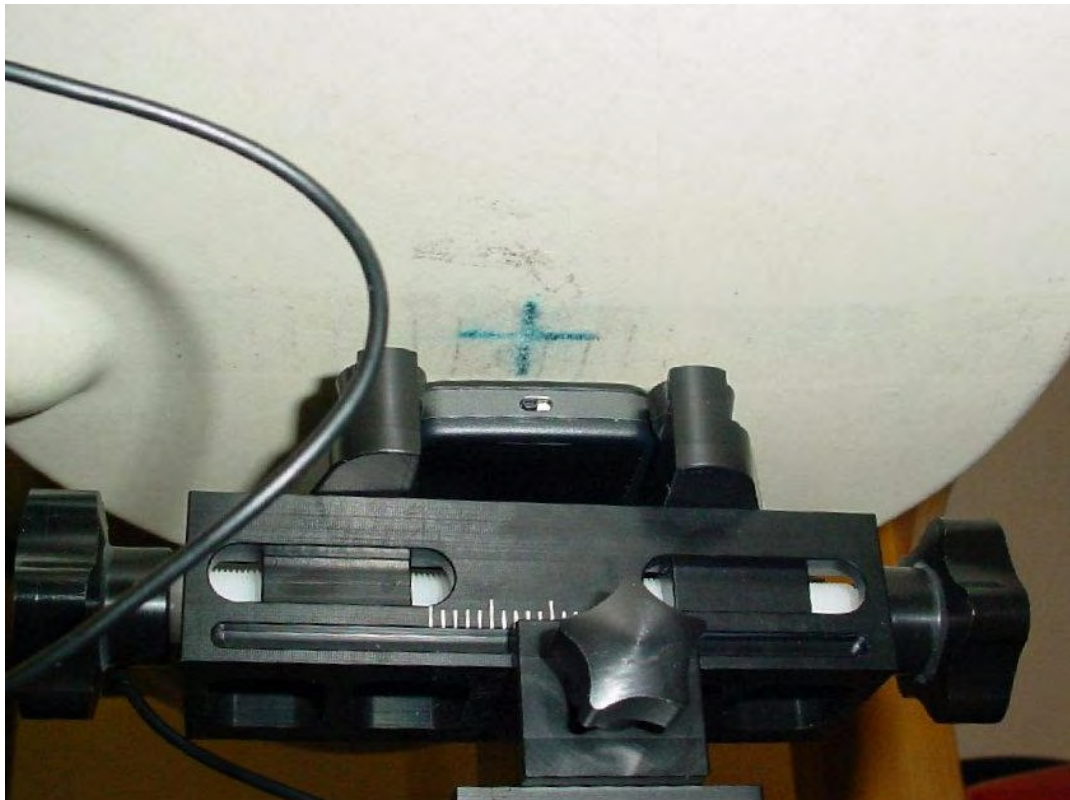
Photo 22: Test position body worn rear side with 15 mm distance
