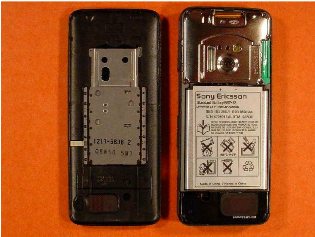
Photo 6: DUT - rear view (open) without battery
