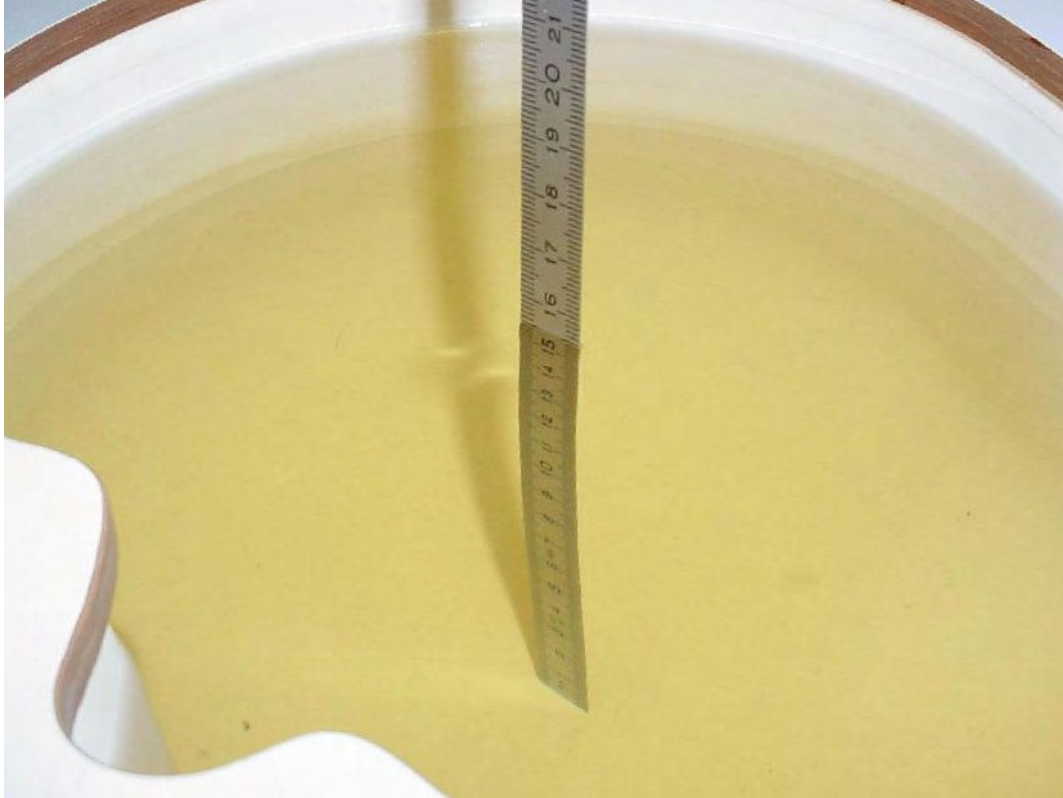
Photo 24: Liquid depth 850 MHz body simulating liquid
