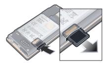
Remove the battery cover and press the edge of the memory card to release and remove it.
