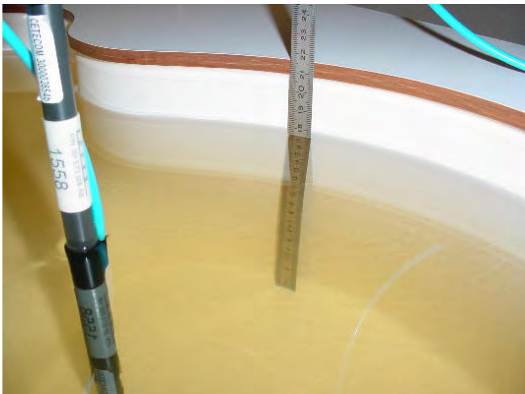
Photo 37: Liquid depth 850 MHz body simulating liquid
