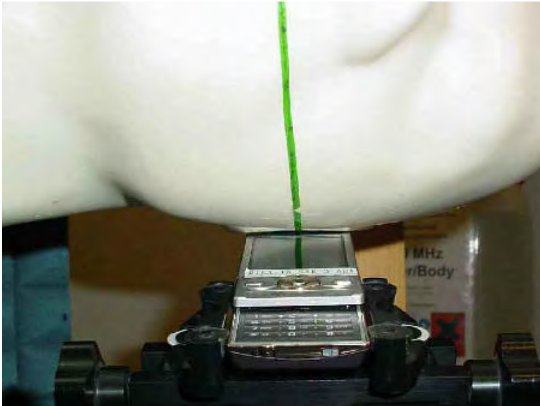
Photo 22: Test position left hand tilted 15° (slide opened)
