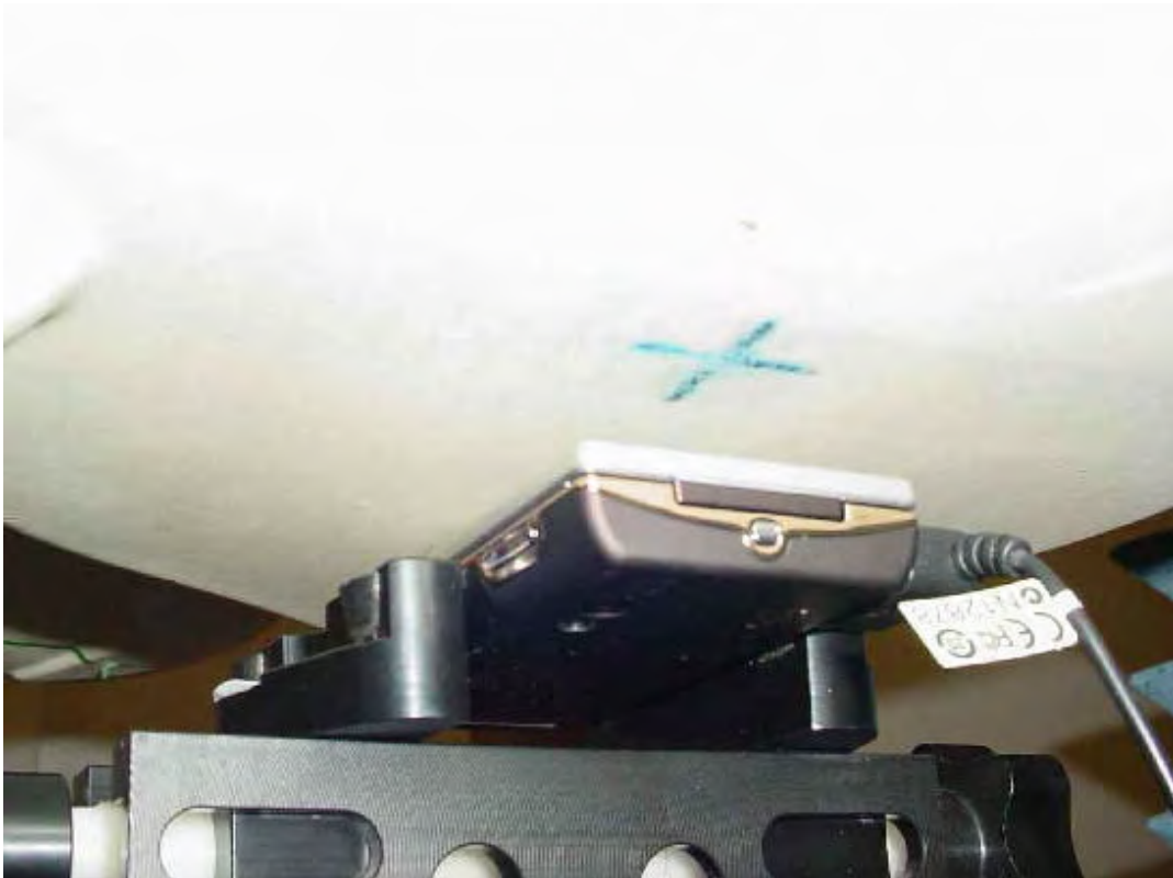
Photo 34: Test position body worn front side (15 mm distance)
