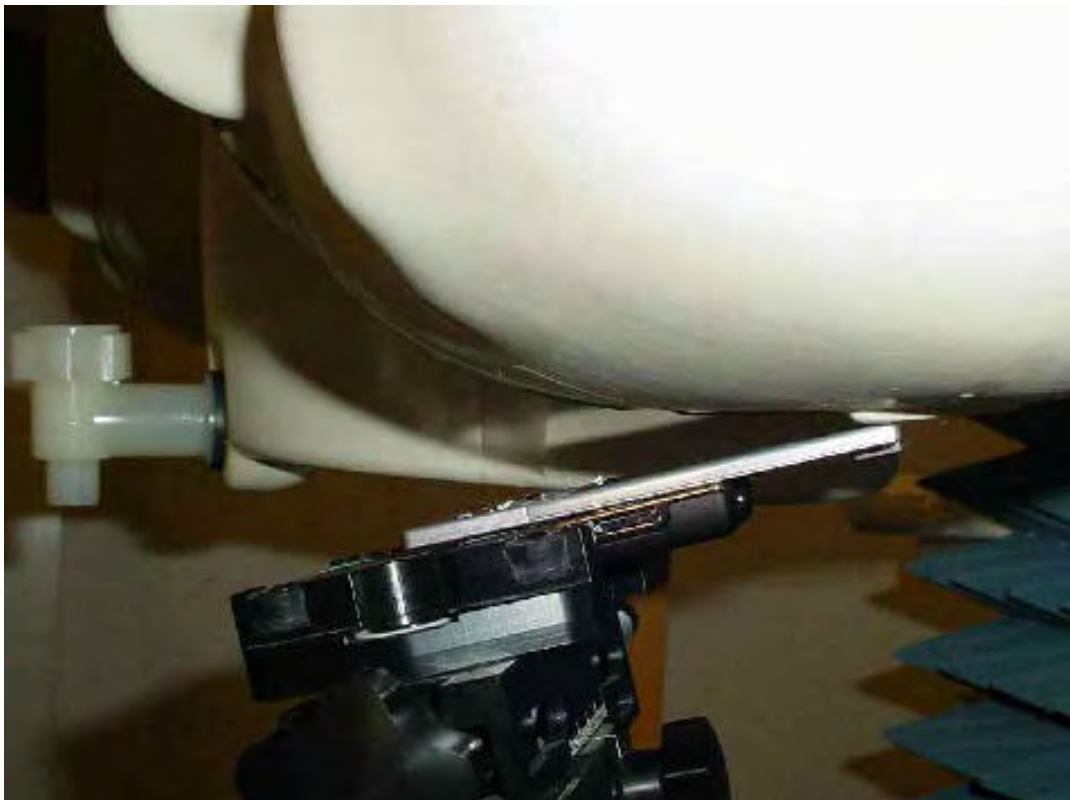
Photo 22: Test position left hand tilted 15° (slide opened)
