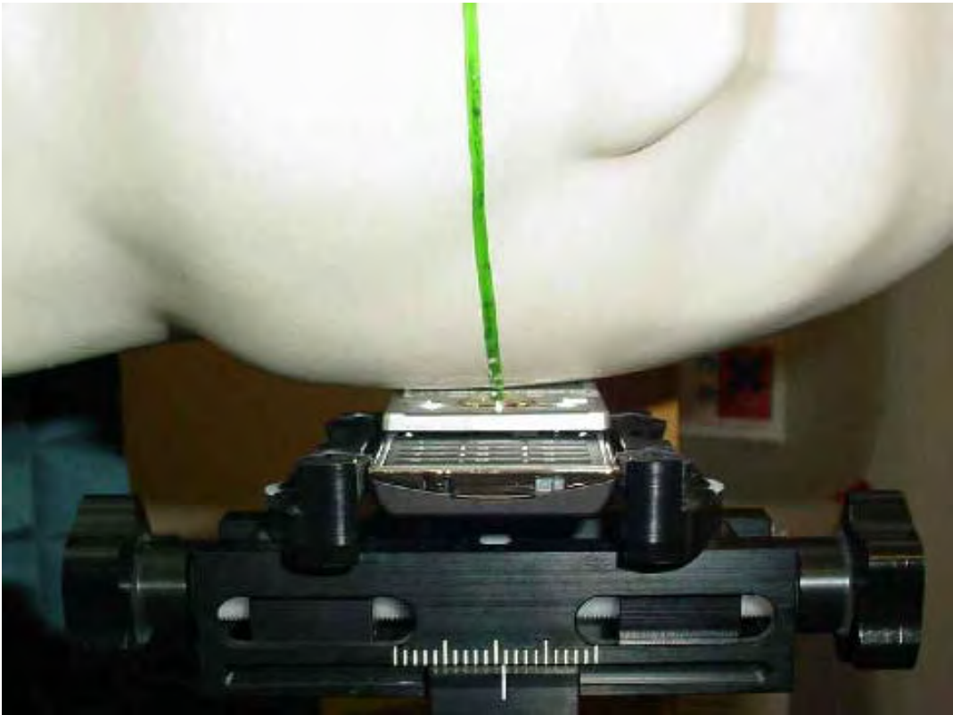
Photo 18: Test position left hand touched (slide opened)
