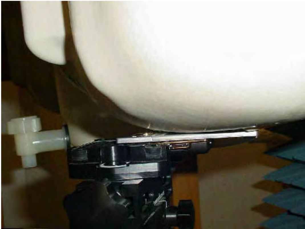
Photo 20: Test position left hand touched (slide opened)
