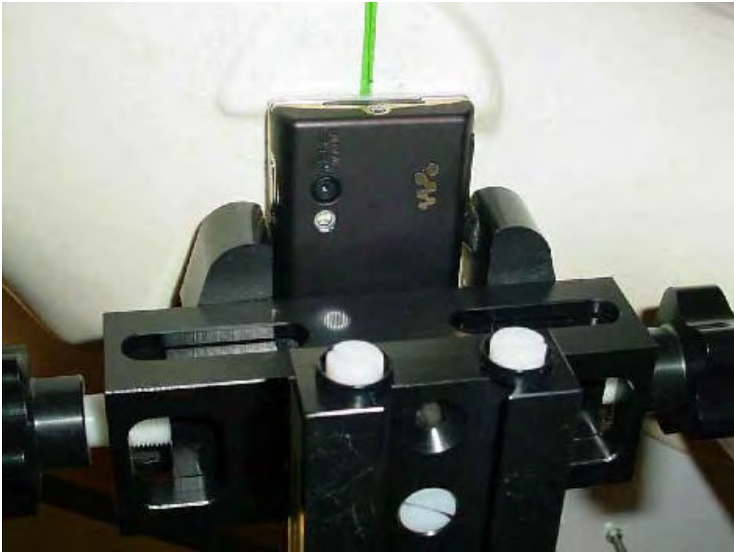
Photo 16: Test position left hand tilted 15° (slide in)
