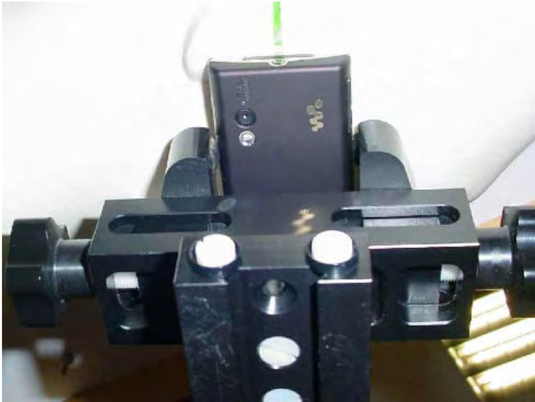
Photo 26: Test position right hand tilted 15° (slide in)
