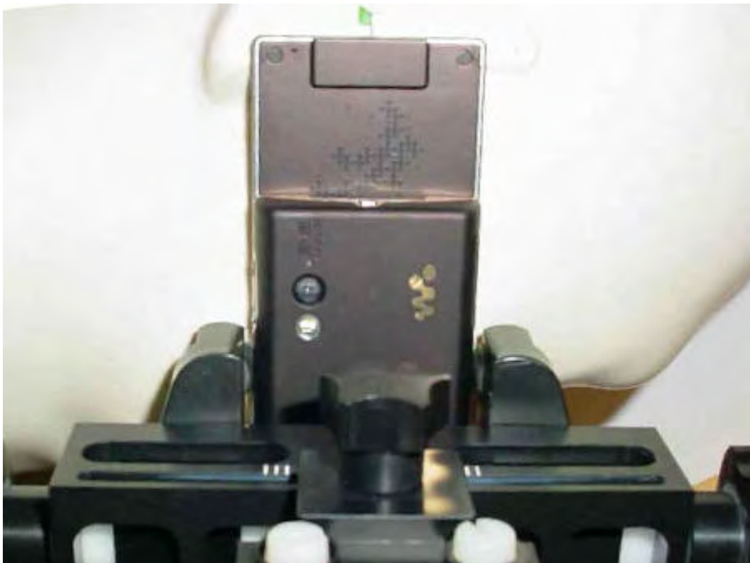
Photo 30: Test position right hand touched (slide opened)
