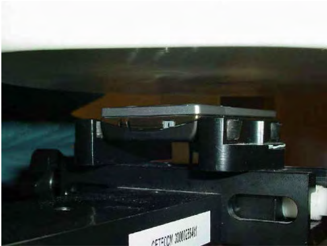
Photo 34: Test position body worn front side (15 mm distance)
