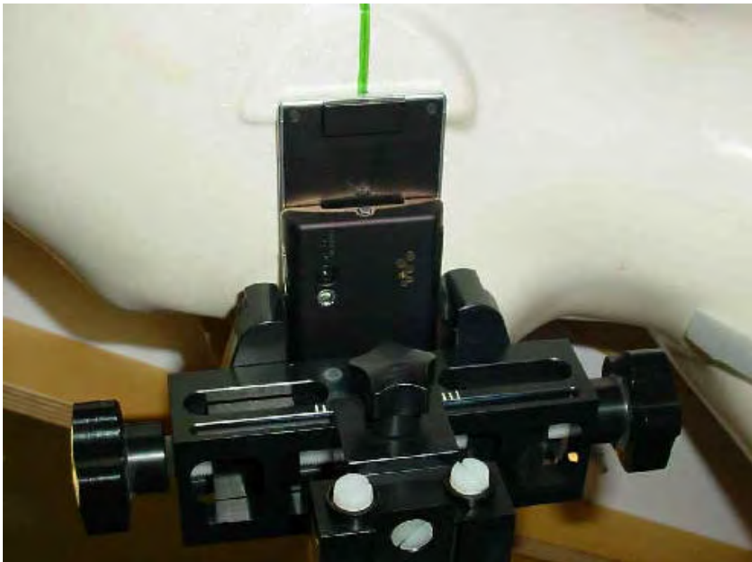
Photo 20: Test position left hand touched (slide opened)
