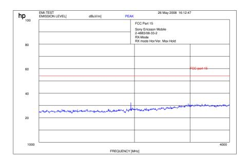
$f < 1 \text{ GHz}: \text{RBW / VBW}: 100 \text{ kHz} \qquad \qquad f \geq 1 \text{GHz}: \text{RBW / VBW}: 1 \text{ MHz}$
