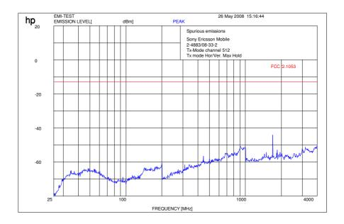
f < 1 GHz : RBW / VBW: 100 kHz Carrier suppressed with a rejection filter  $f \ge 1GHz : RBW / VBW:1 MHz$
