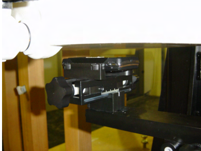
DUT in body position with 15 mm distance
