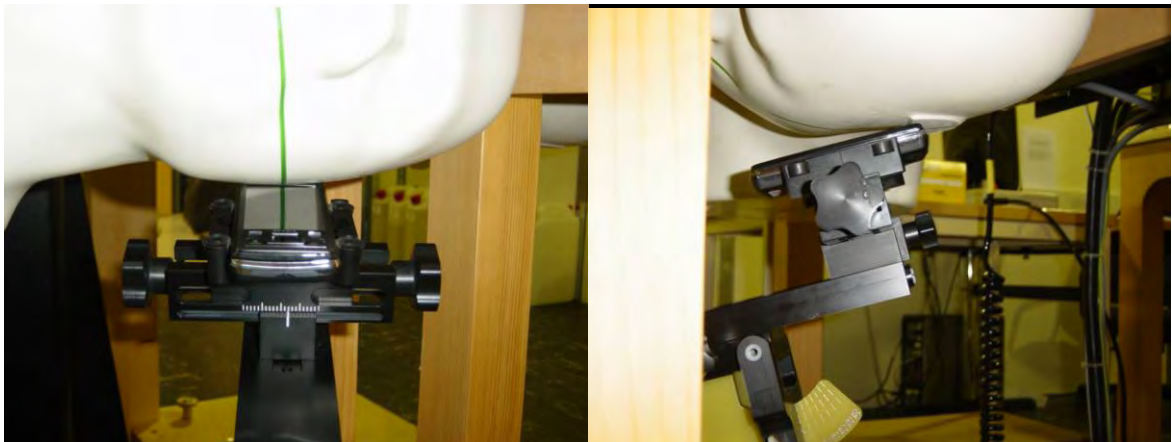
DUT position towards the head: Tilt (touch + 15°) position
