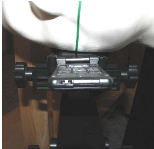
DUT position towards the head: Cheek (touch) position
