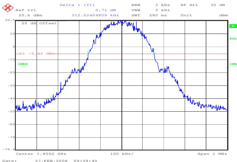
**Channel 661****99% (-20 dB) Occupied Bandwidth**
