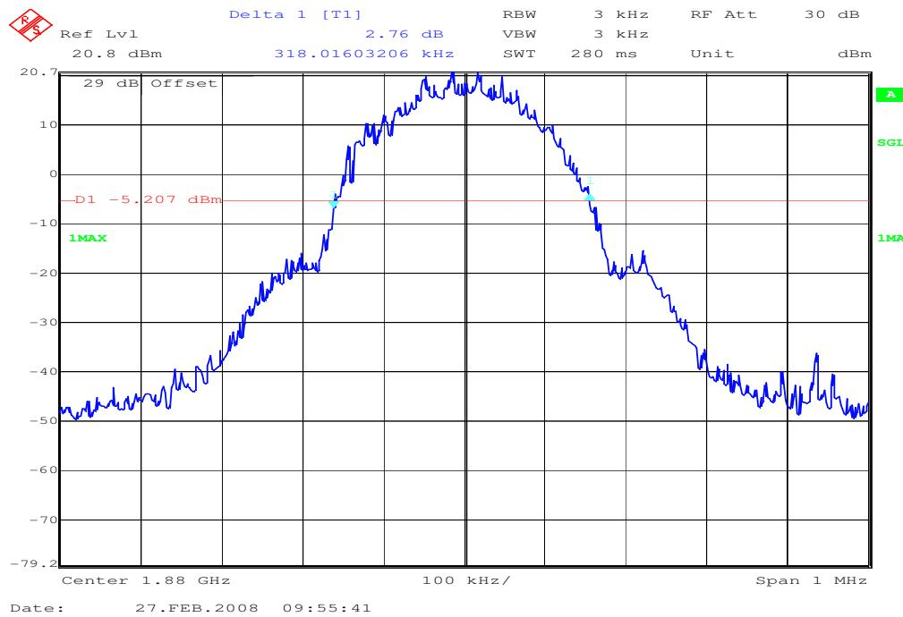
**Channel 810****99% (-20 dB) Occupied Bandwidth**
