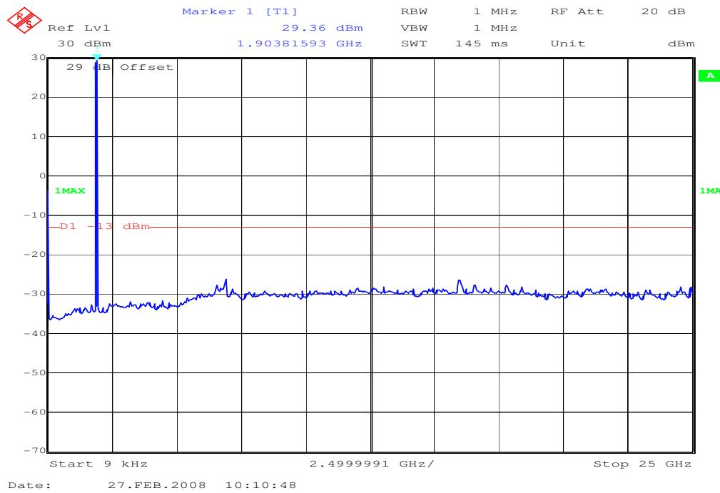
The peak at the beginning of the plot at 9 kHz is the LO (local oscillator) from our spectrum analyzer.
