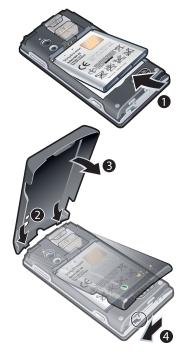
1 Insert the battery with the label side up and the connectors facing each other.
