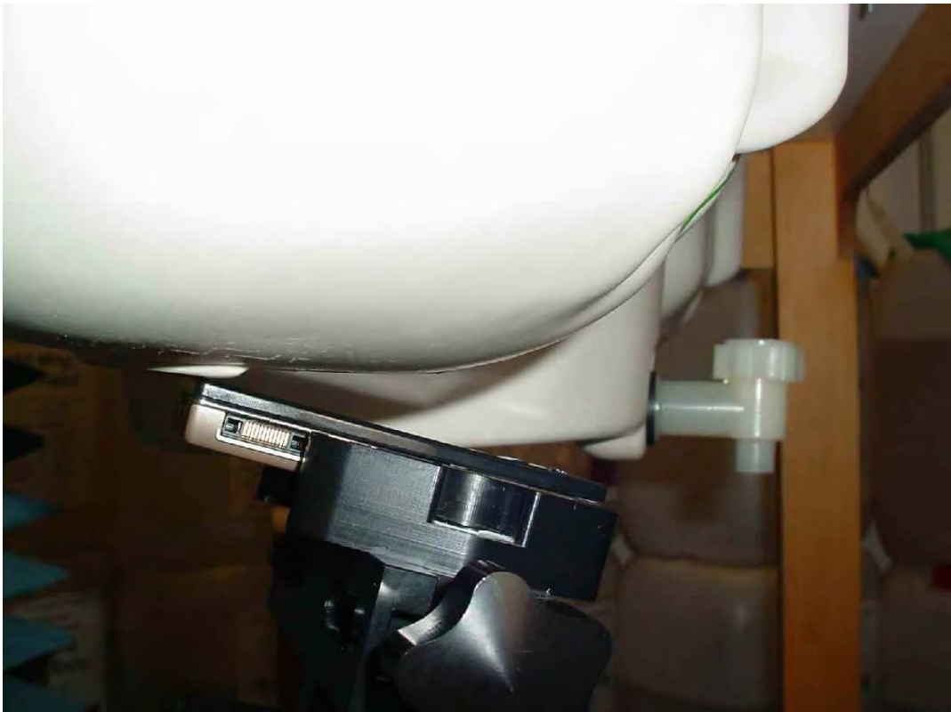
Photo 26: Test position right hand tilted 15° (slide-in)
