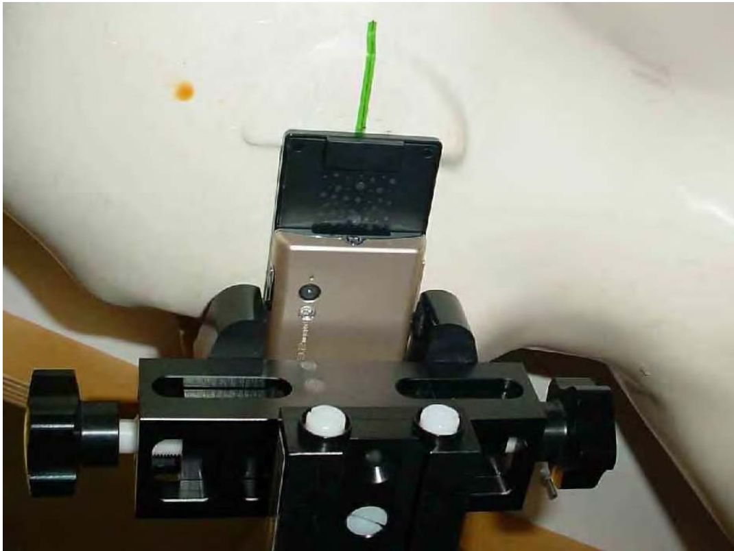
Photo 20: Test position left hand tilted 15° (slide opened)
