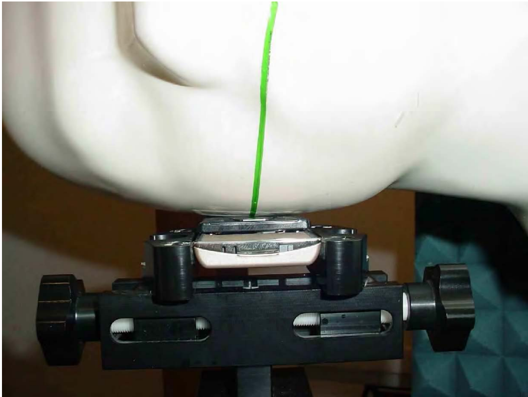
Photo 28: Test position right hand touched (slide opened)
