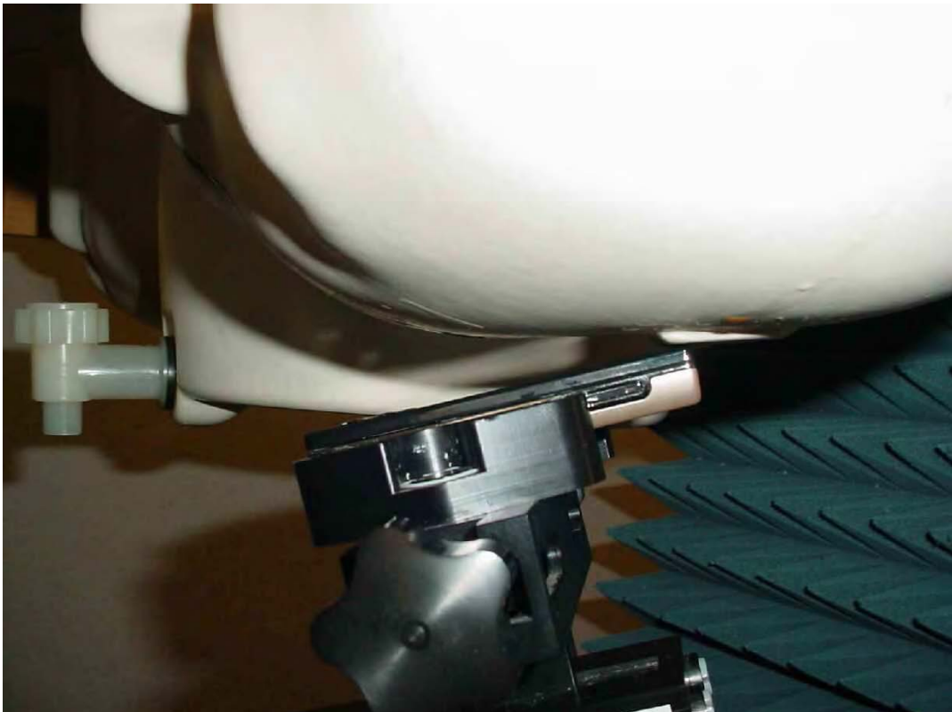
Photo 16: Test position left hand tilted 15° (slide-in)
