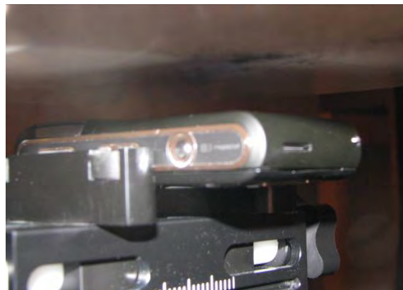
DUT position towards the body with a maximum distance of 15 mm
