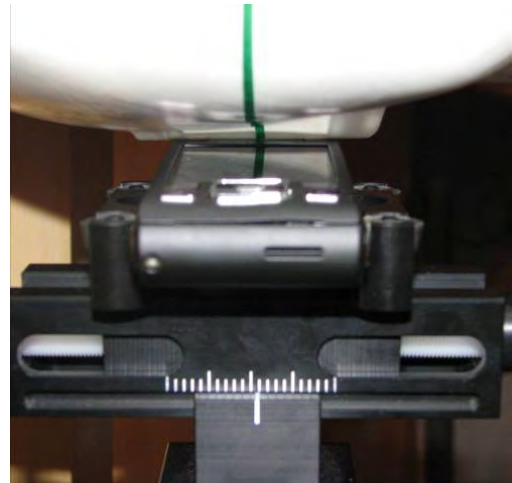
DUT position towards the head: Tilt (touch + 15°) position
