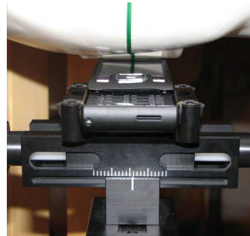
DUT position towards the head with camera cover extracted: Tilt
