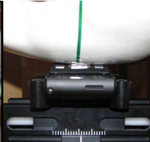
DUT position towards the head with camera cover extracted: Cheek
