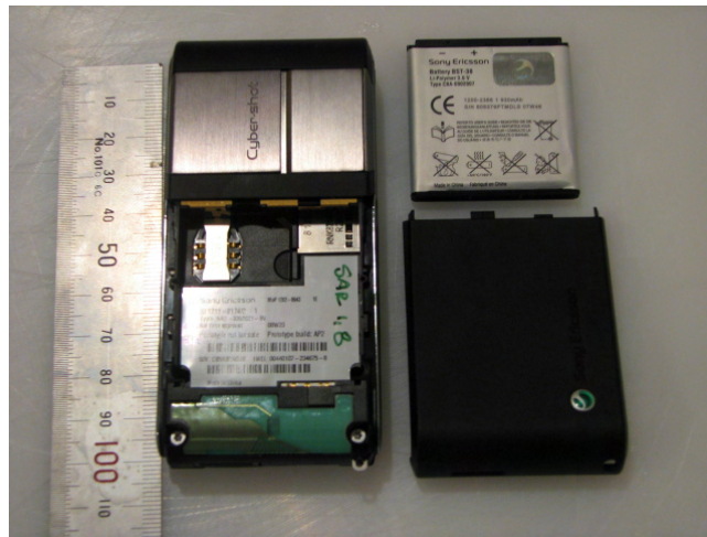
Battery and cover removed
