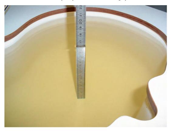
Photo 37: Liquid depth 850 MHz body simulating liquid
