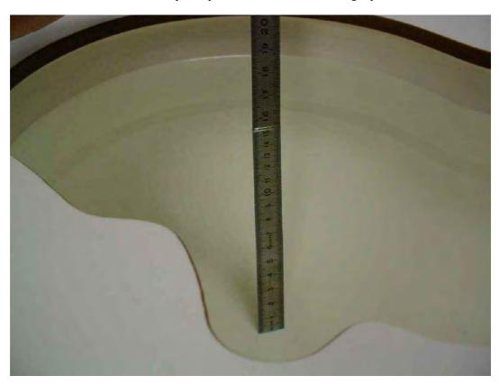
Photo 39: Liquid depth 1900 MHz body simulating liquid
