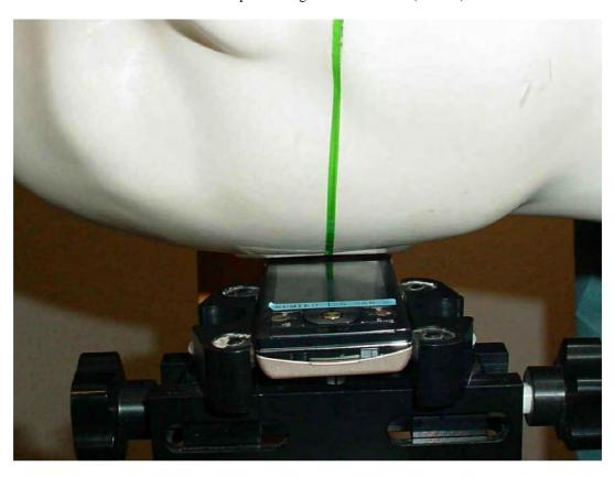
Photo 26: Test position right hand tilted  $15^{\circ}$  (slide in)
