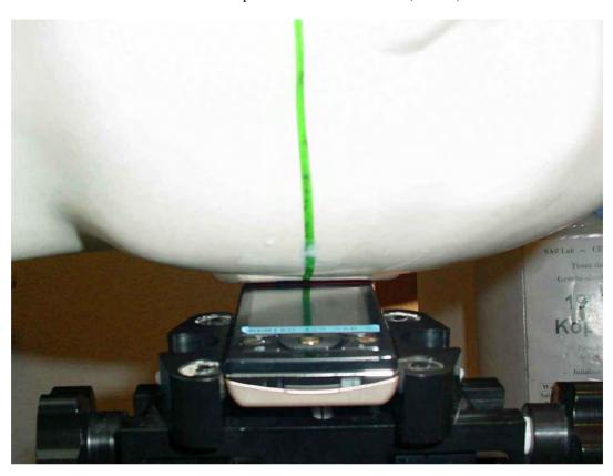
Photo 16: Test position left hand tilted 15° (slide in)
