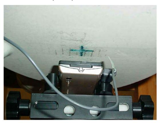
Photo 34: Test position body worn rear side with 15 mm distance
