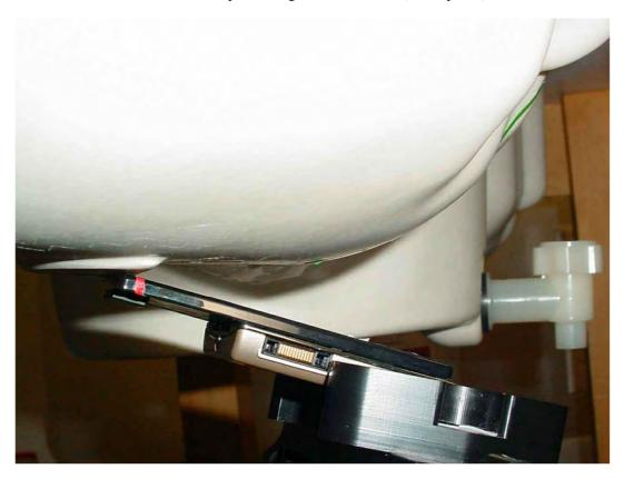
Photo 32: Test position body worn front side with 15 mm distance
