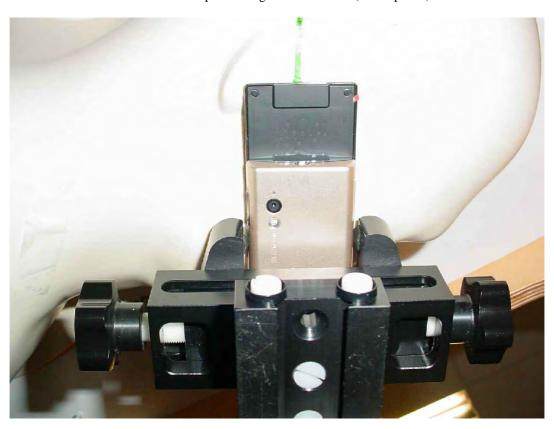
Photo 30: Test position right hand tilted 15° (slide opened)
