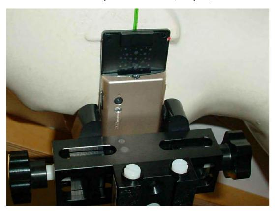
Photo 20: Test position left hand tilted 15° (slide opened)
