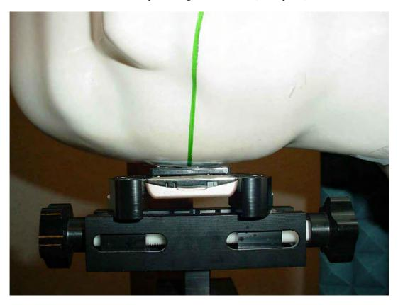
Photo 28: Test position right hand touched (slide opened)
