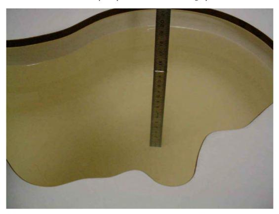
Photo 41: Liquid depth 2450 MHz body simulating liquid
