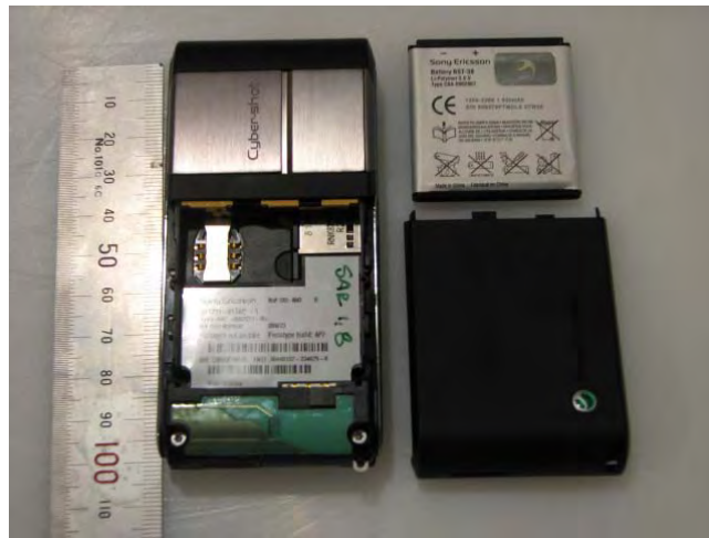
Battery and cover removed
