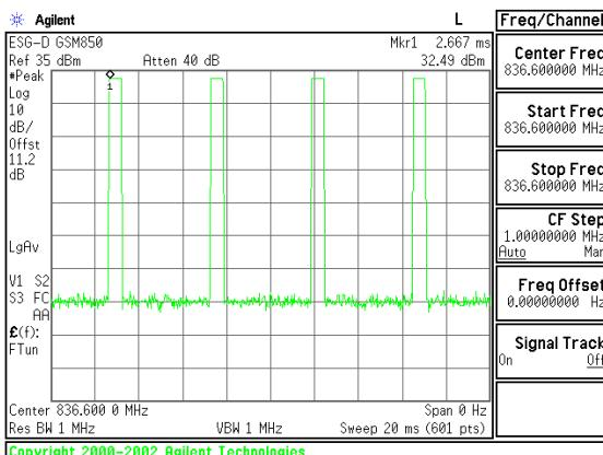
Figure 8-4 GSM850 Signal
