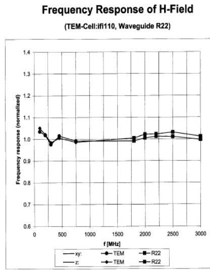
**Figure 5-4 H-Field Probe Frequency Response**
