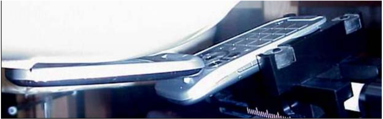
Position of device against head phantom using the “cheek” position
