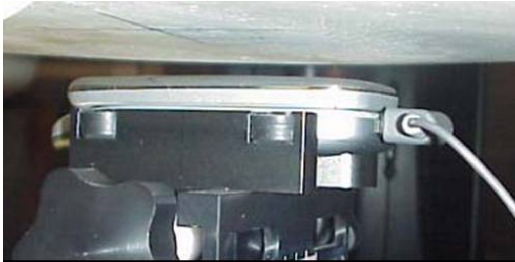
Position with front of device against flat phantom using a 15mm SPACER with hands free accessory.
