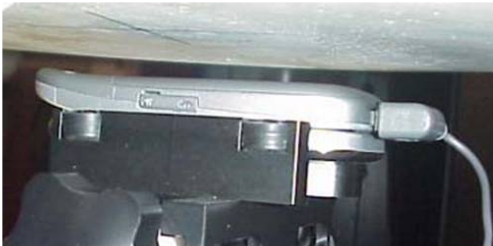
Position with back of device against flat phantom using a 15mm SPACER with hands free accessory.
