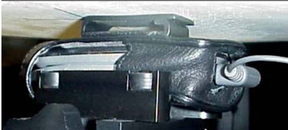
Position with front of device against flat phantom using an ICE26 carry case with hands free accessory.
