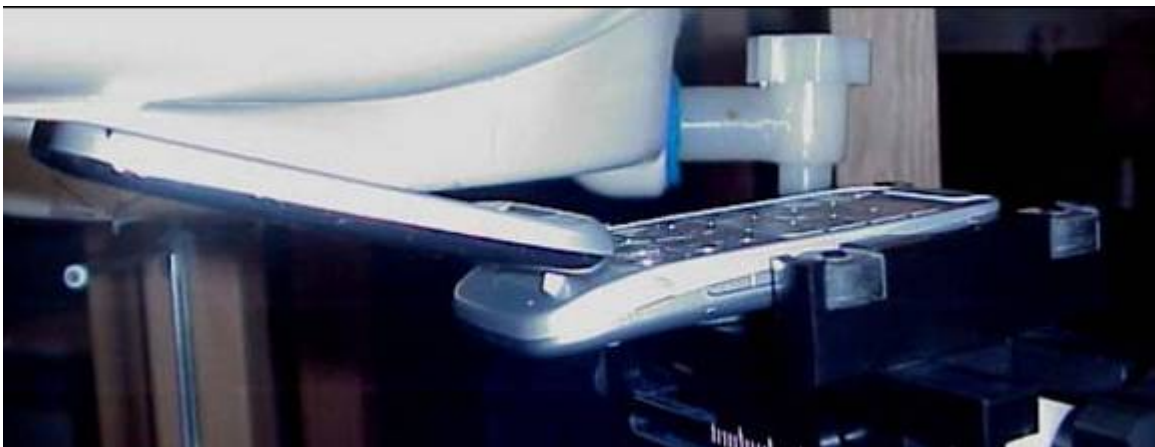
Position of device against head phantom using the “tilt” position
