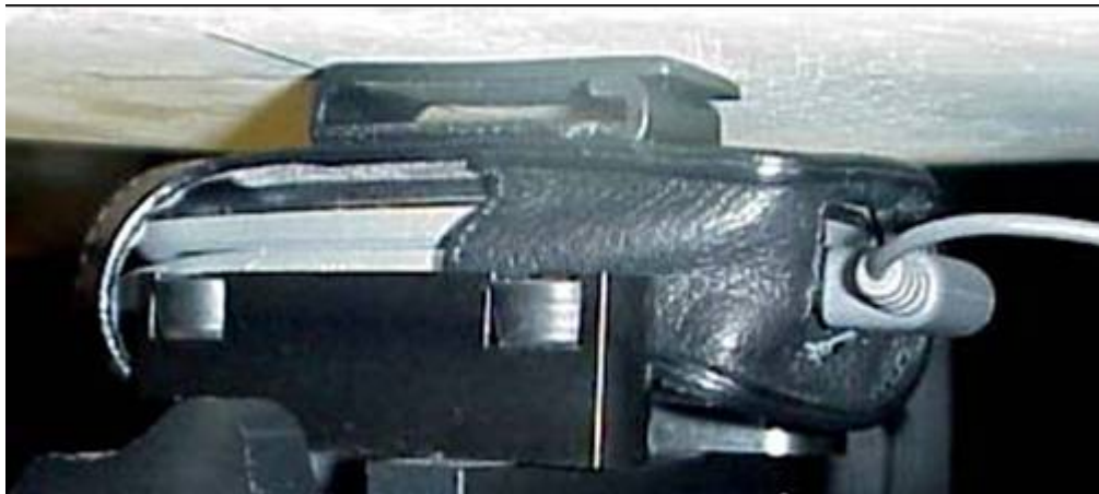
Position with back of device against flat phantom using an ICE26 carry case with hands free accessory.
