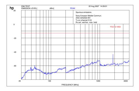
f < 1 GHz : RBW/VBW: 100 kHz f > 1 GHz : RBW / VBW 1 MHz Carrier suppressed with a rejection filter
