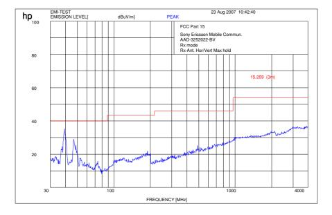
$\label{eq:generalized_formula} \begin{array}{l} f < 1 \ \mathrm{GHz} : \mathrm{RBW/VBW} : 100 \ \mathrm{kHz} \\ f > 1 \ \mathrm{GHz} : \mathrm{RBW} \ / \ \mathrm{VBW} \ 1 \ \mathrm{MHz} \end{array}$
