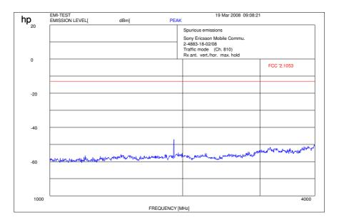
$f \ge 1$ GHz: RBW / VBW 1 MHz Carrier suppressed with a rejection filter
