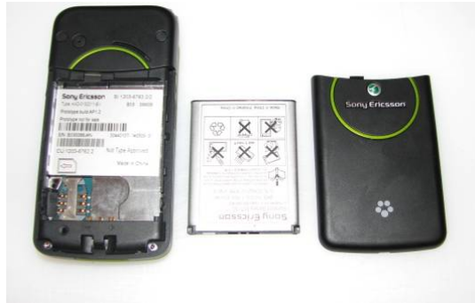
Battery and cover removed
