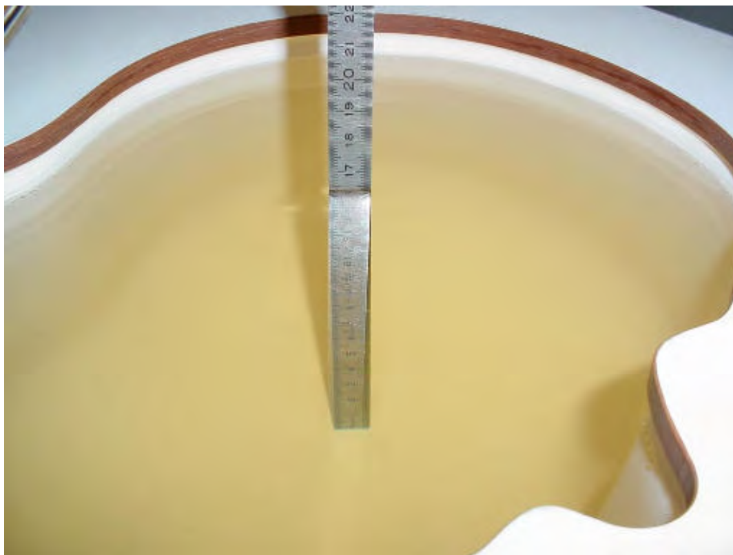
Photo 37: Liquid depth 850 MHz body simulating liquid
