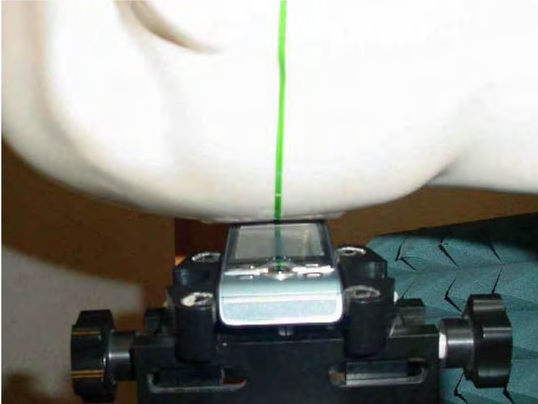
Photo 26: Test position right hand tilted 15°
