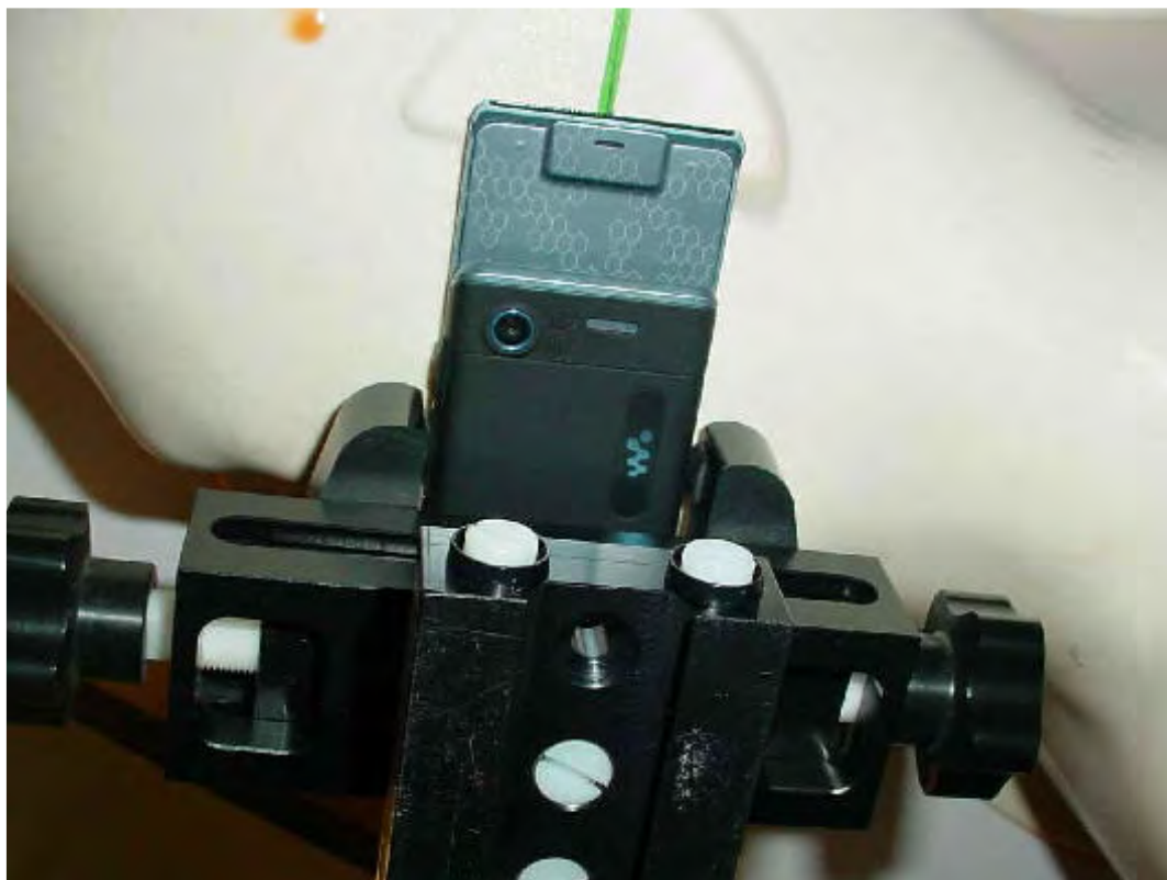
Photo 20: Test position left hand tilted 15° slide opened
