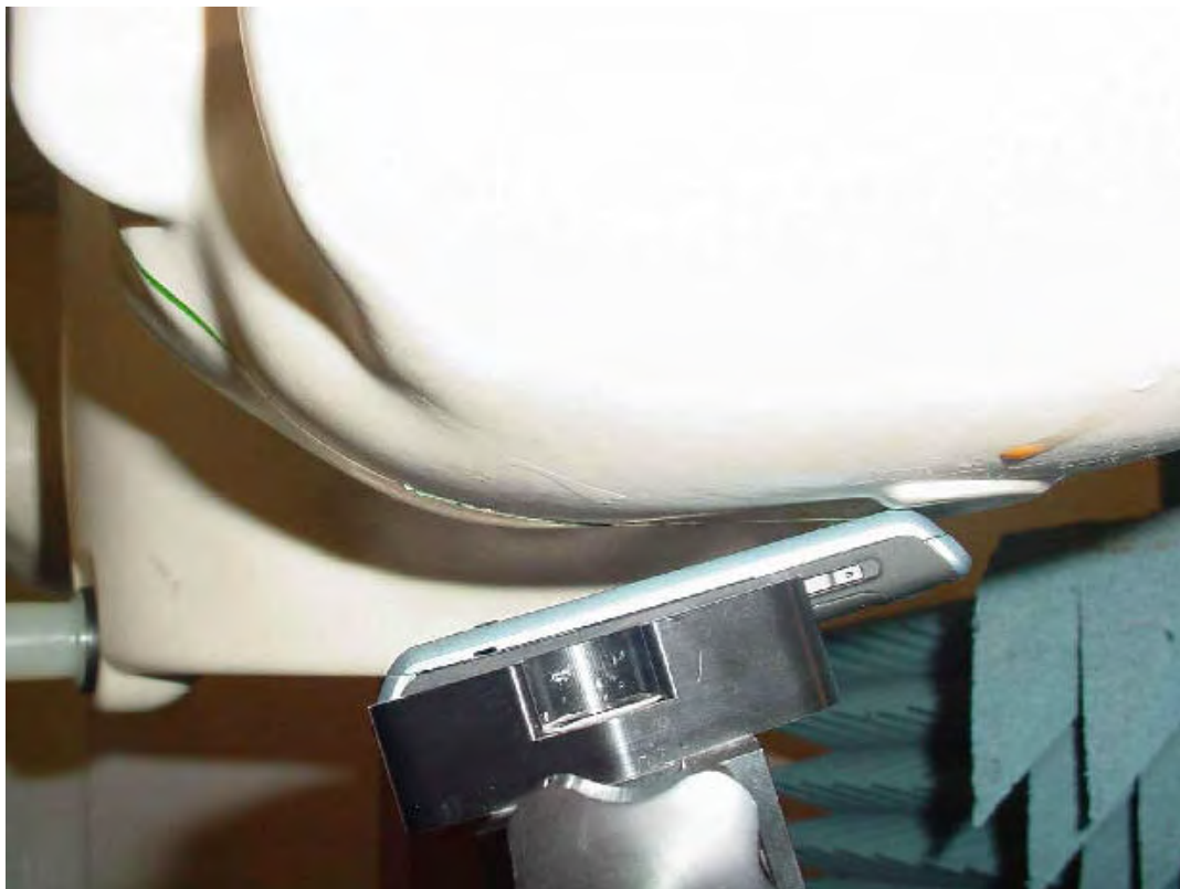
Photo 16: Test position left hand tilted 15°
