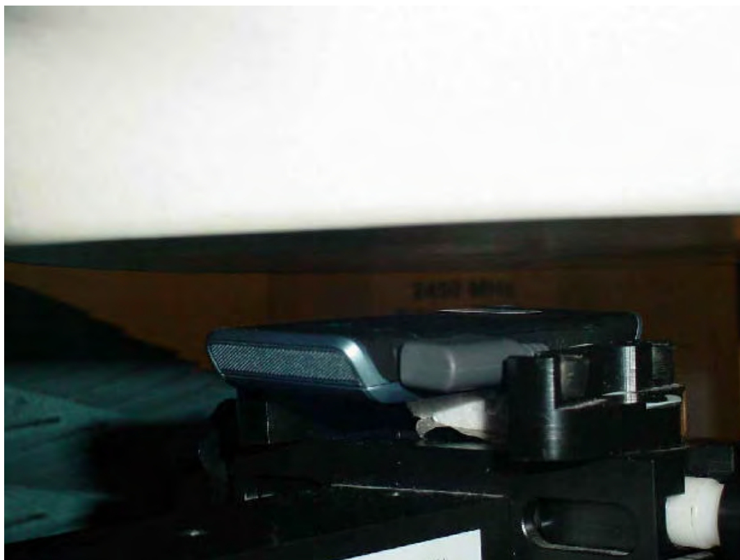
Photo 35: Test position body worn rear side (15 mm distance)
