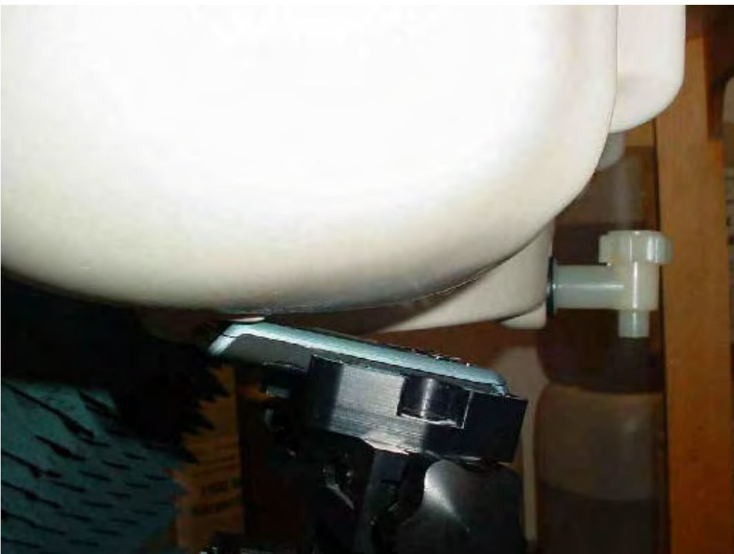
Photo 26: Test position right hand tilted 15°
