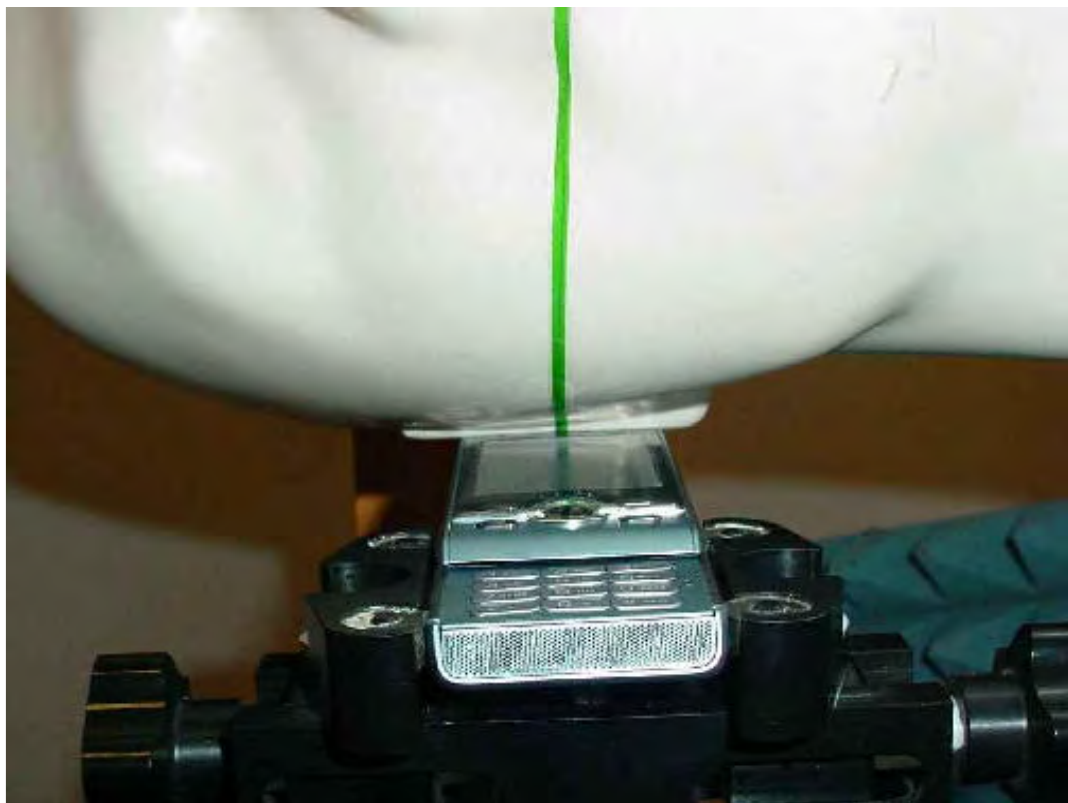
Photo 30: Test position right hand tilted 15° slide opened
