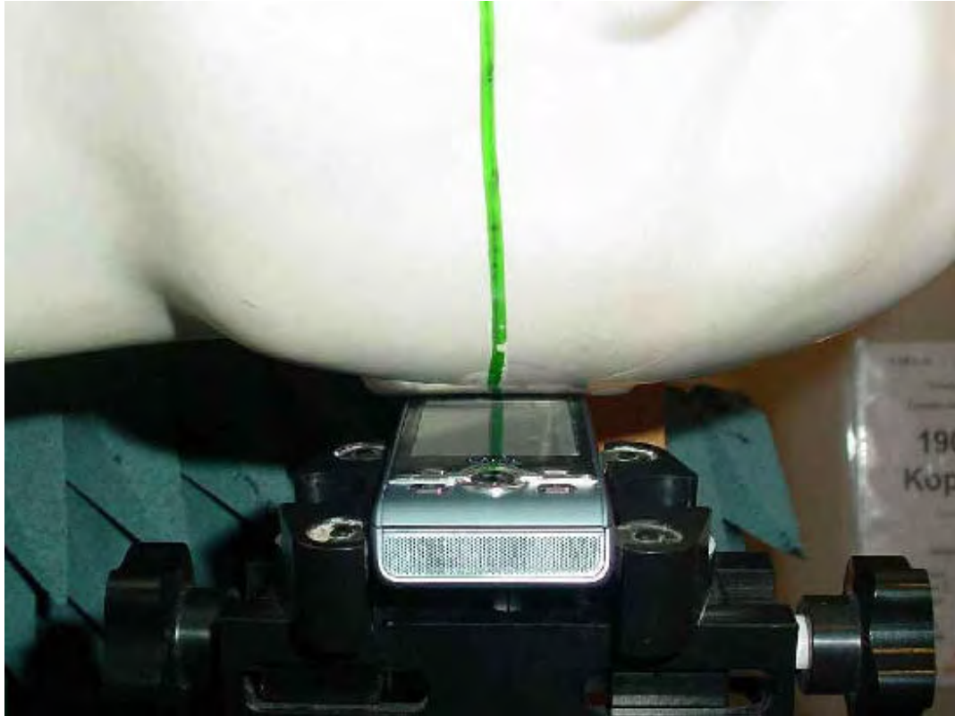
Photo 16: Test position left hand tilted 15°
