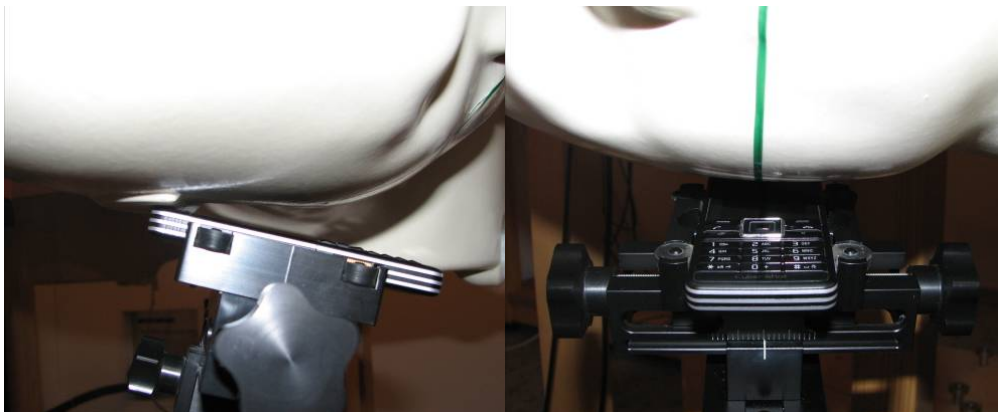
DUT position towards the head: Tilt (touch + 15°) position
