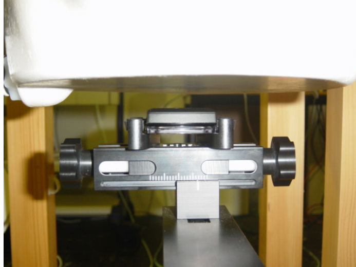
DUT in body position with 15 mm distance
