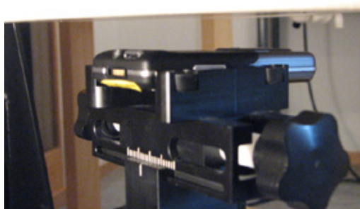
Device position against the body: Phone on 15mm distance against Phantom
