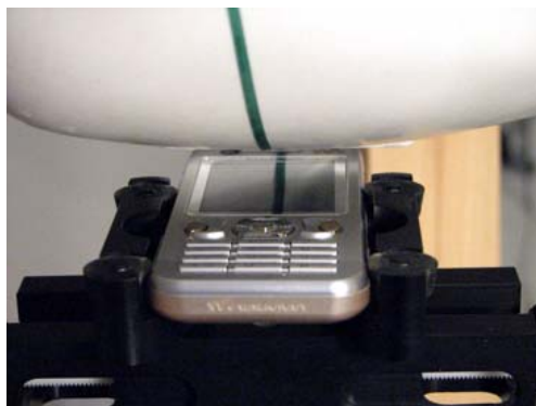
Device position towards the head: Tilt (cheek+15deg) phone position
