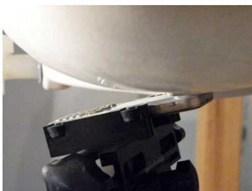
Device position towards the head: Tilt (cheek+15deg) phone position
