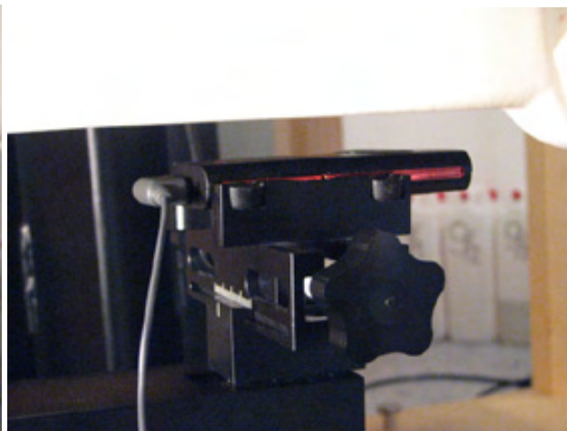
Device position against the body: 15mm distance from Phantom.
