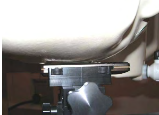
DUT position towards the head: Cheek (touch) position
