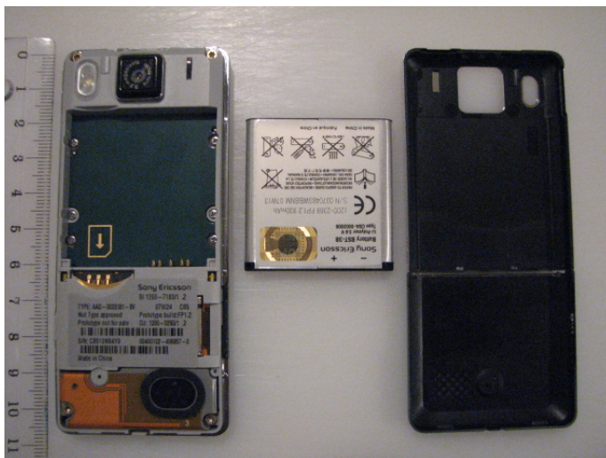
Battery and batterycover removed
