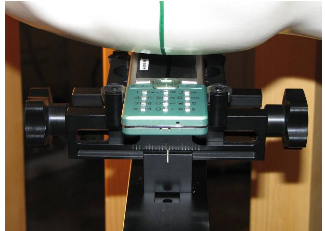
DUT position towards the head: Tilt (touch + 15°) phone position
