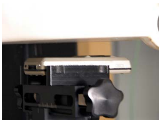
Device position against the body: Phone on 15mm distance against Phantom
