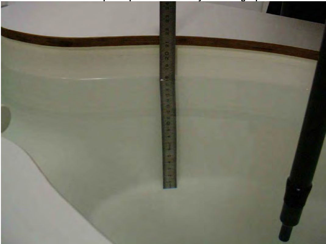
Photo 6: Liquid depth 2450 MHz body simulating liquid
