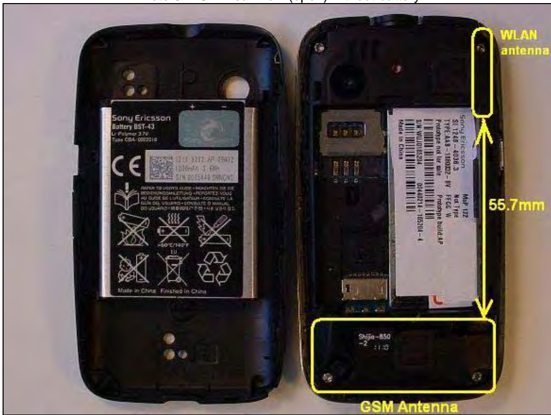
Photo 6: DUT - rear view (open) without battery
