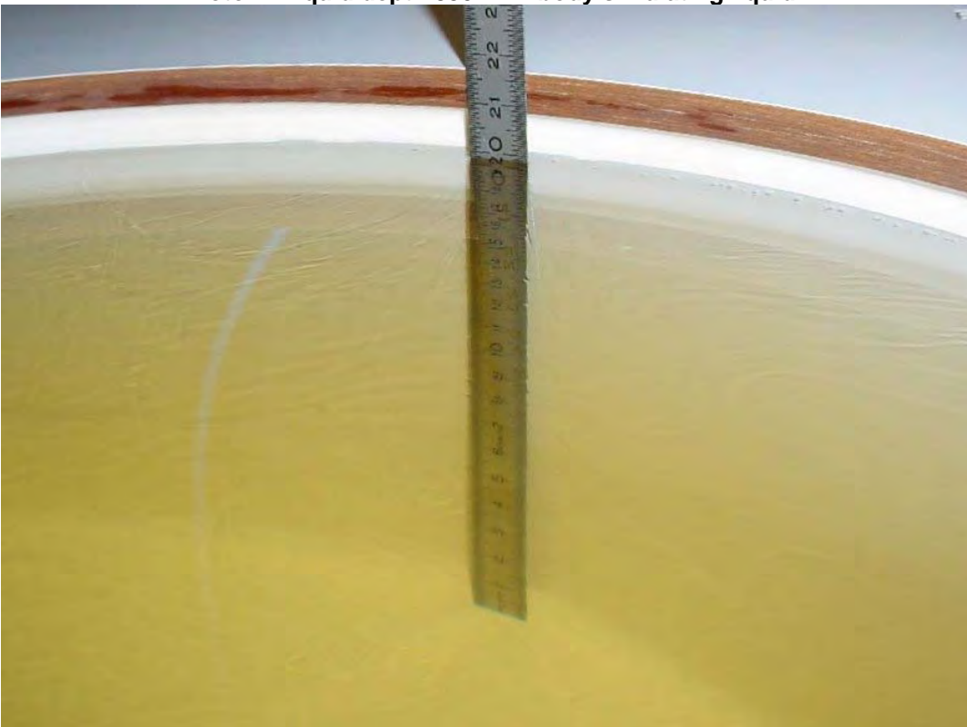
Photo 2: Liquid depth 850 MHz body simulating liquid
