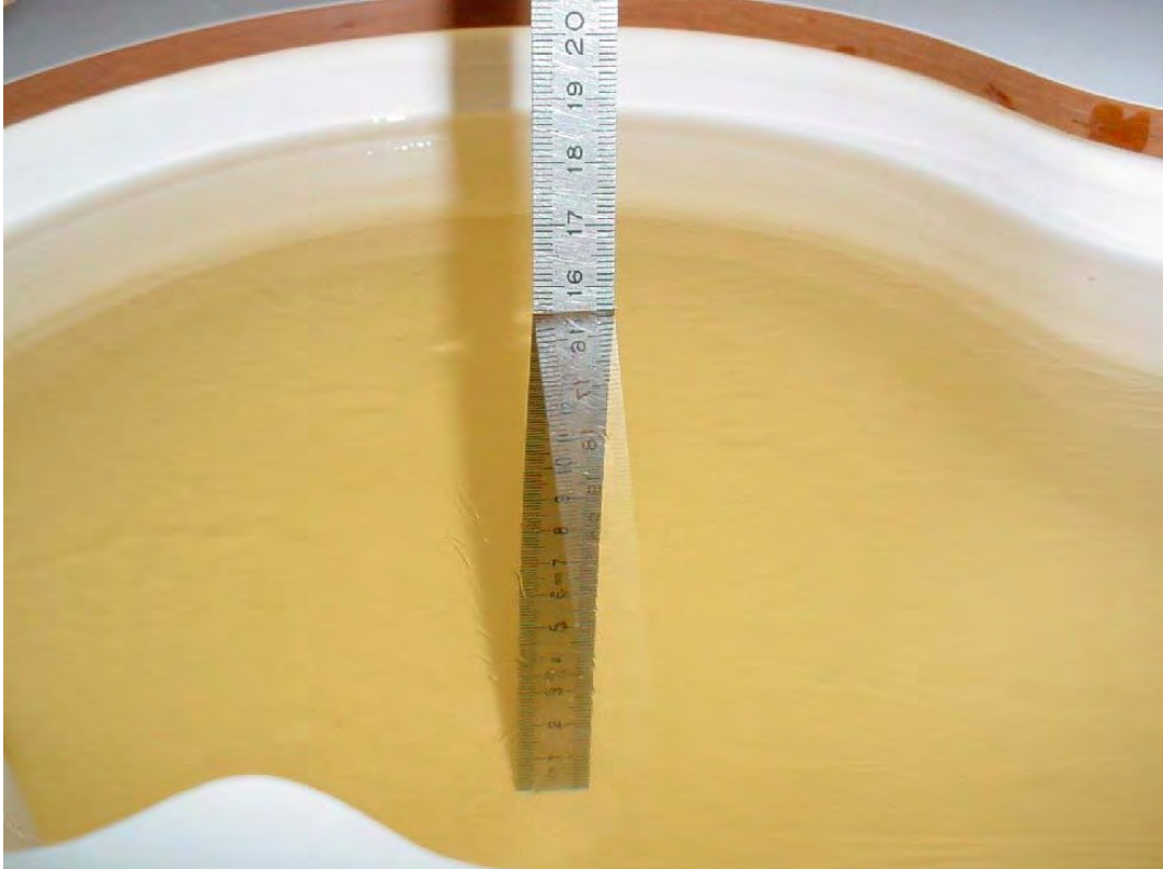
Photo 2: Liquid depth 850 MHz body simulating liquid
