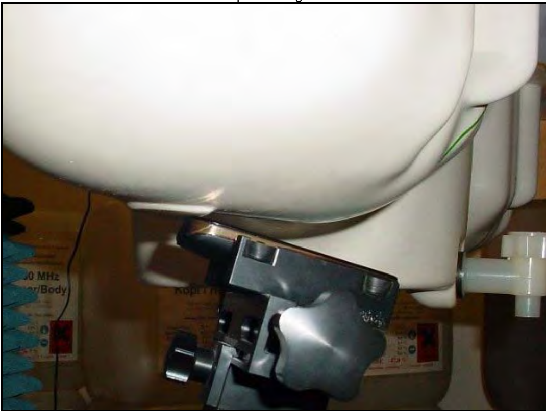
Photo 18: Test position right hand tilted 15°
