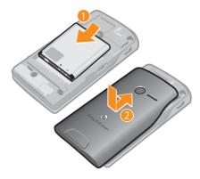
1 Insert the battery with connectors facing each other. 2 Attach the battery cover.
