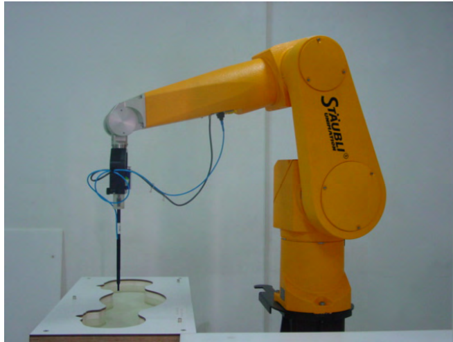
Picture B1: Specific Absorption Rate Test Layout
