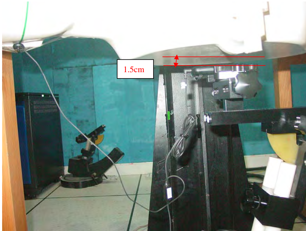
Picture G12: Body-worn Position with headset (EUT towards ground, the distance from handset to the bottom of the Phantom is 1.5cm) – Slide down
