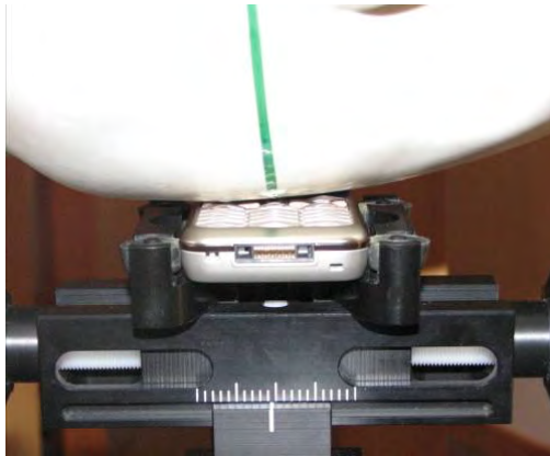
DUT position towards the head: Cheek (touch) position
