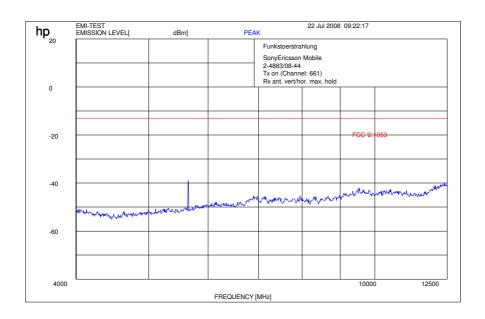
$f < 1 \text{ GHz}: \text{RBW/VBW}: 100 \text{ kHz} \qquad \qquad f \geq 1 \text{GHz}: \text{RBW/VBW} \text{ 1 MHz}$
