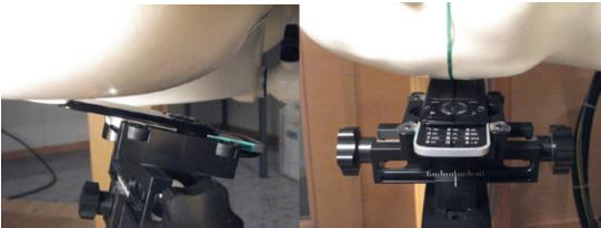
DUT position towards the head: Tilt (touch + 15°) position open
