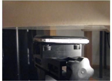
DUT in body position with 15 mm distance
