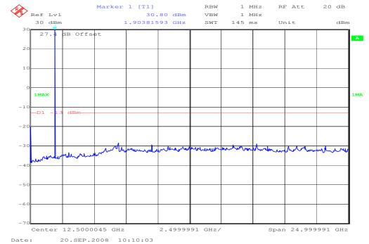
The peak at the beginning of the Plot is the LO from the measuring spectrum Analyzer and not from the EUT.
