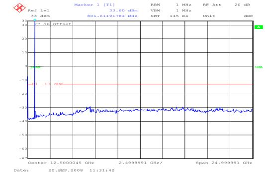
The peak at the beginning of the Plot is the LO from the measuring spectrum Analyzer and not from the EUT.
