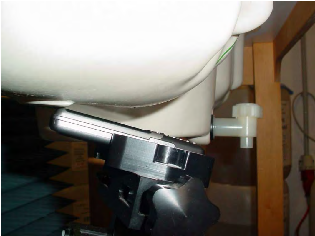
Photo 18: Test position right hand tilted 15°
