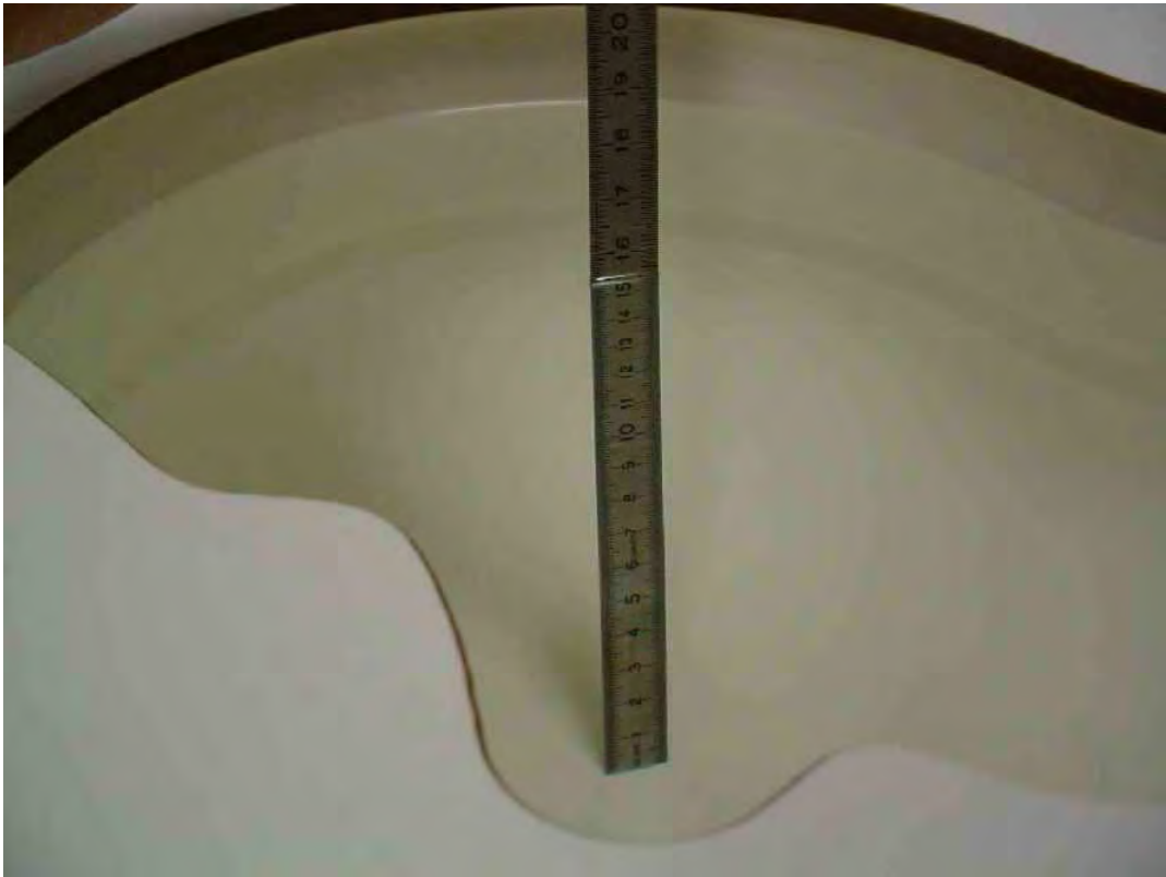
Photo 26: Liquid depth 1900 MHz body simulating liquid
