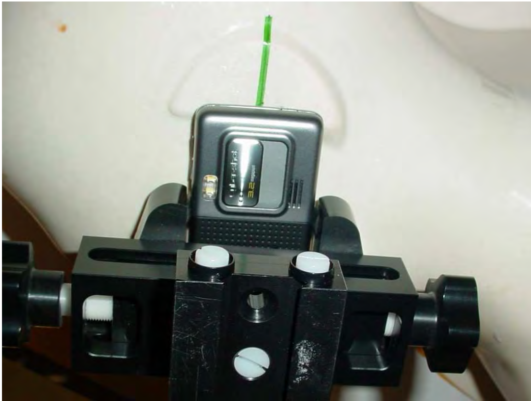
Photo 12: Test position left hand tilted 15°
