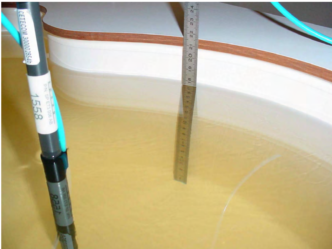
Photo 24: Liquid depth 850 MHz body simulating liquid
