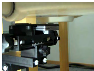
Device position towards the body: Phone on 15mm distance against Phantom
