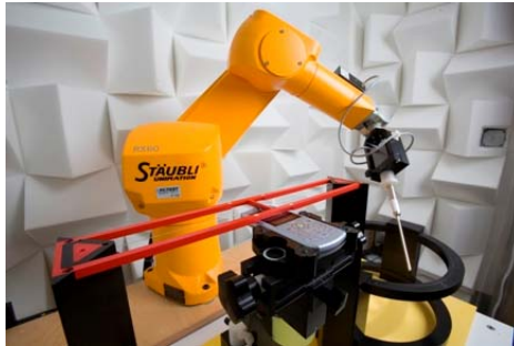
Figure 5-5 SPEAG Robotic System
