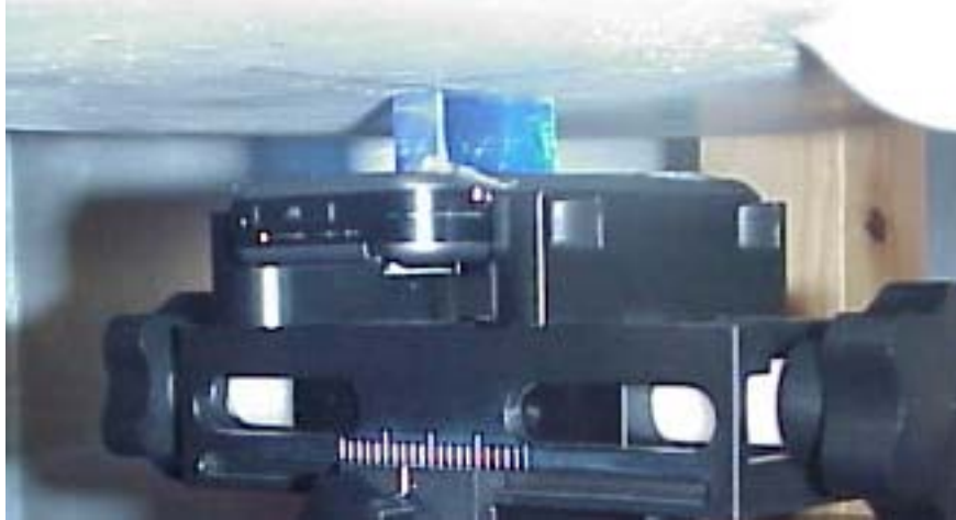
Position with front of device against flat phantom using a 15mm SPACER with hands free accessory.
