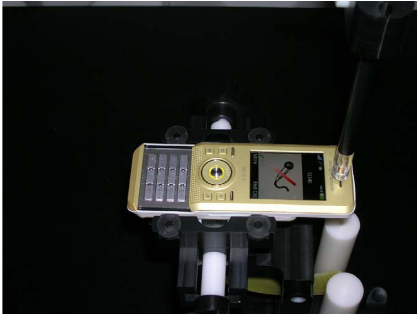
Figure 12-1 Test Setup for Wireless Device
