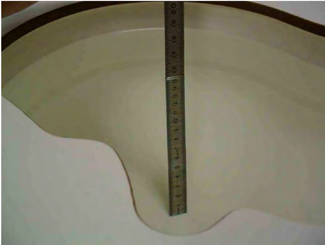
Photo 26: Liquid depth 1900 MHz body simulating liquid
