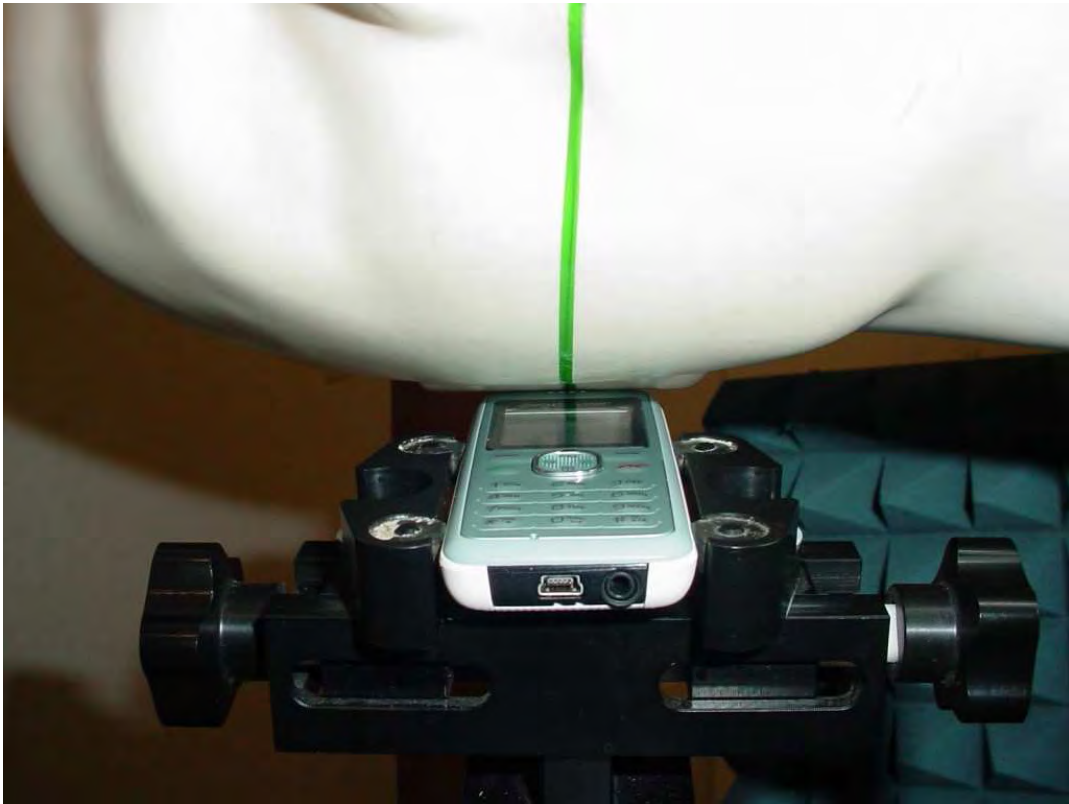
Photo 18: Test position right hand tilted 15°
