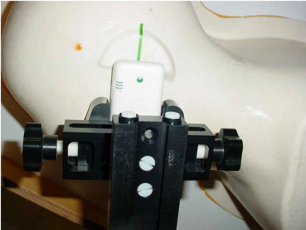
Photo 12: Test position left hand tilted 15°
