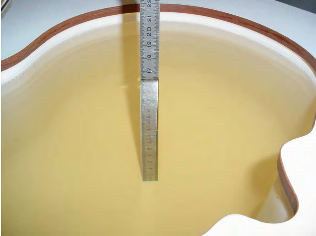
Photo 24: Liquid depth 850 MHz body simulating liquid
