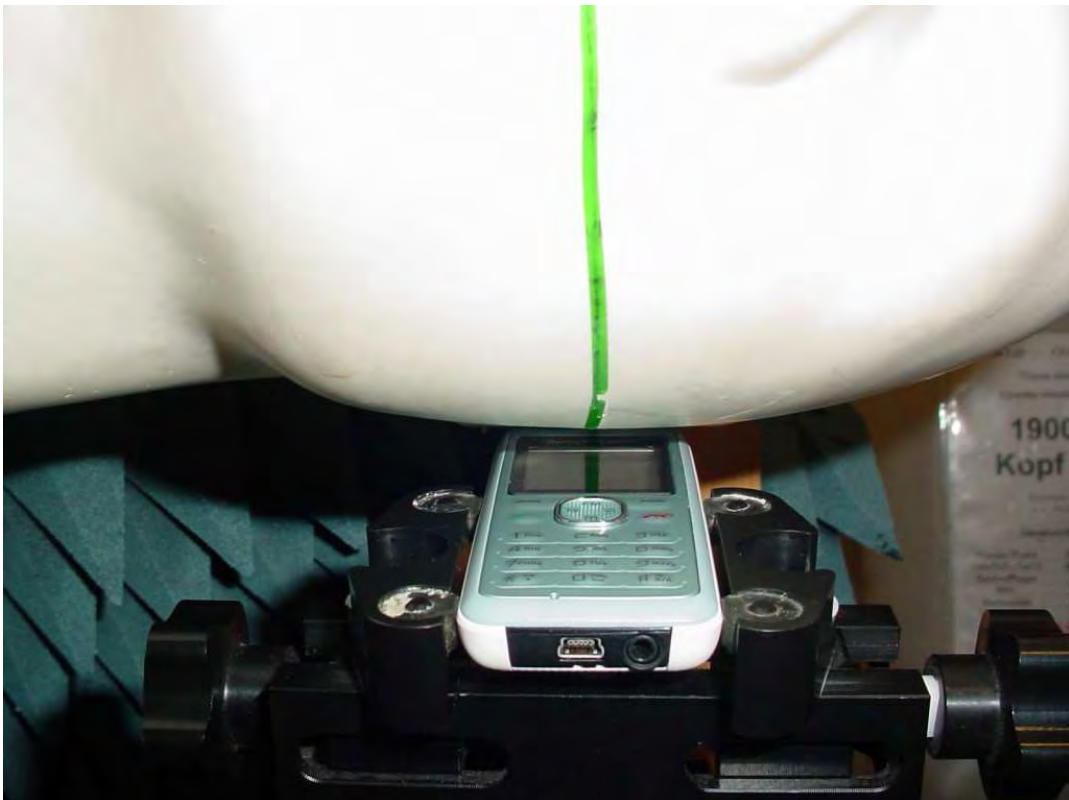
Photo 12: Test position left hand tilted 15°
