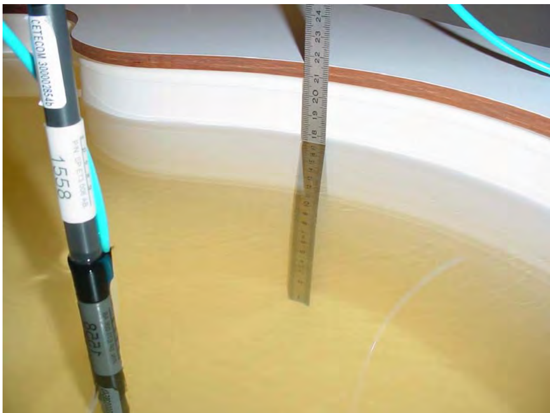
Photo 24: Liquid depth 850 MHz body simulating liquid
