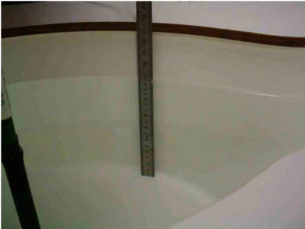
Photo 26: Liquid depth 1900 MHz body simulating liquid
